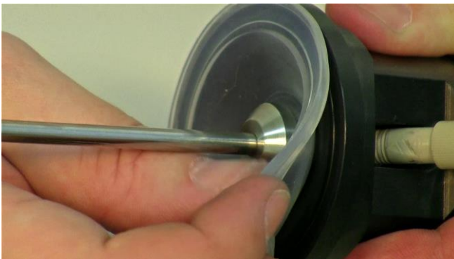
Figure 3.5-19 Ensure that the large silicon sterility membrane is fitted correctly and firmly in the designed grooves on the head of the agitation unit.
