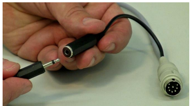
Figure 3.14—24 Plug in the DOZITO's black cable to the black cable of ANTIFO, as shown.
