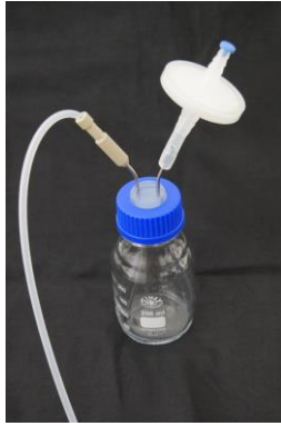
Figure 3.12-1 Intermediary bottle between air condenser and outlet filter
