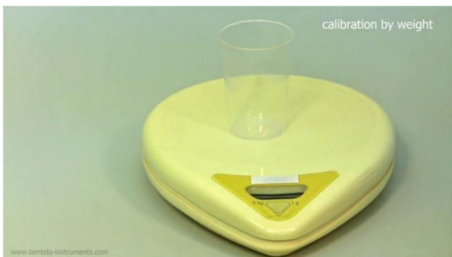
Figure 5.4—6 Measure the weight of the empty beaker using a sensitive weighing scale. For the exact measurement of the liquid collected, tare the weighing scale with the measuring beaker (Example: 0.000 g).
