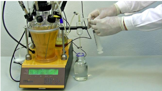
Figure 8.2—1 Open the clamp on the tubing that connects the syringe.
