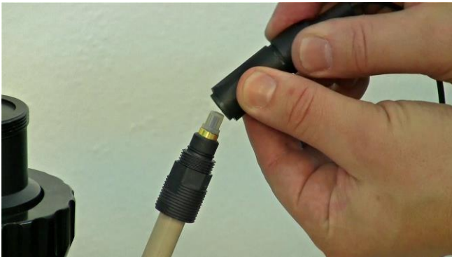
Figure 3.7-11 pO 2 (DO) probe connector have to be connected between the pO 2 probe and the pO 2 (DO) probe socket in the base control unit. Adjust the sleeve of the pO 2 (DO) probe connector by pushing it up as shown.
