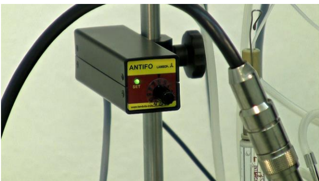
Figure 3.14—1 ANTIFO (foam detector and controller). Place the main body of the ANTIFO on one of the support rods of the MINIFOR laboratory fermenter/bioreactor (e.g. under a pump carrying support). In this way, it will be accessible and occupy minimal space.
