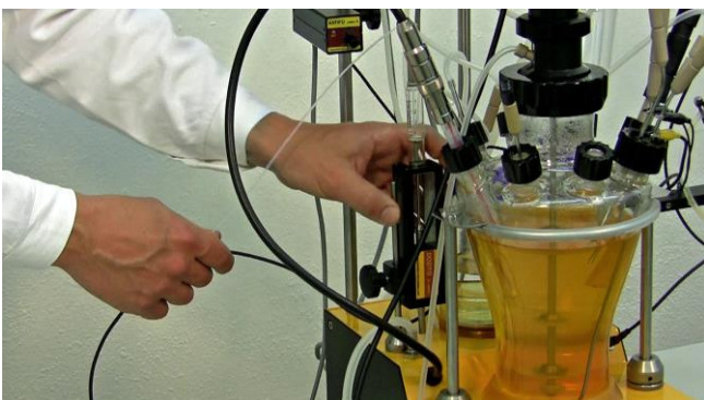
Figure 3.14—23 Place the DOZITO on the MINIFOR base unit with the help of the magnetic stand in DOZITO.
