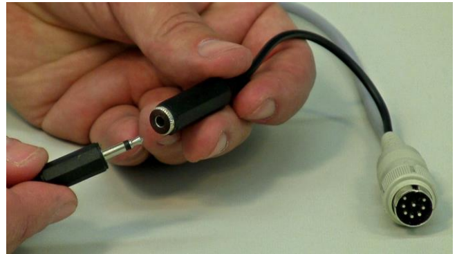
Figure 3.15—32 Plug in the DOZITO's black cable to the black cable of ANTIFO, as shown.
