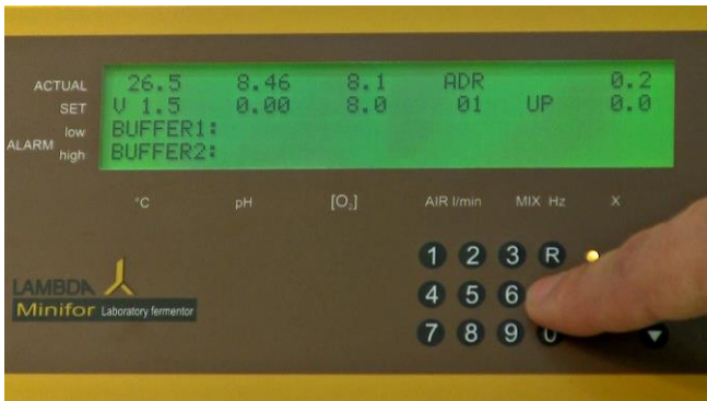
Figure 5.3—7 Press the calibration key "C". The calibrated value will be shown as BUFFER 1 value of [O 2 ].
