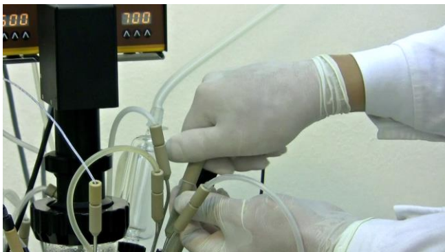
Figure 8.2—1 As a first step, loosen the septum protection cap.
