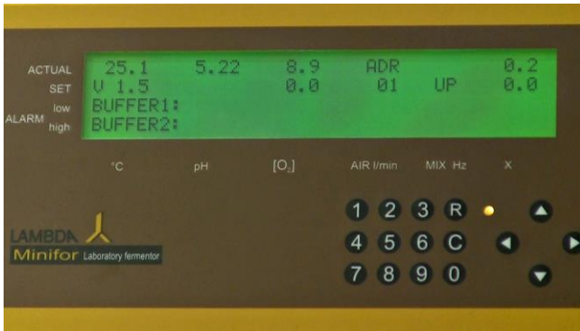
Figure 4.2—3 Calibration mode - Key "C" starts the calibration of pH, pO 2 , parameter X or the setting of the address for PC control (depending on the choice with the cursor). The LED is yellow and the regulation is off. (Only the agitation is activated to allow precise calibration of pO 2 probe).
