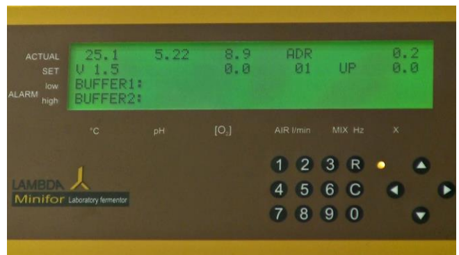
Figure 4.1—5 The cursor is represented by the blinking of the activated digit.
