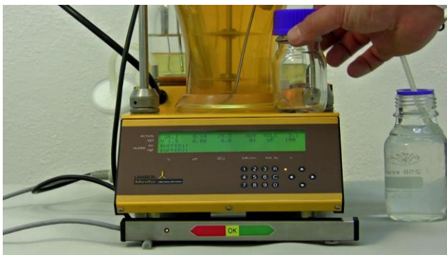
Figure 5.5—9 Then place a known weight or add a certain known volume of liquid to the glass bottle. Say 100 g or ml.
