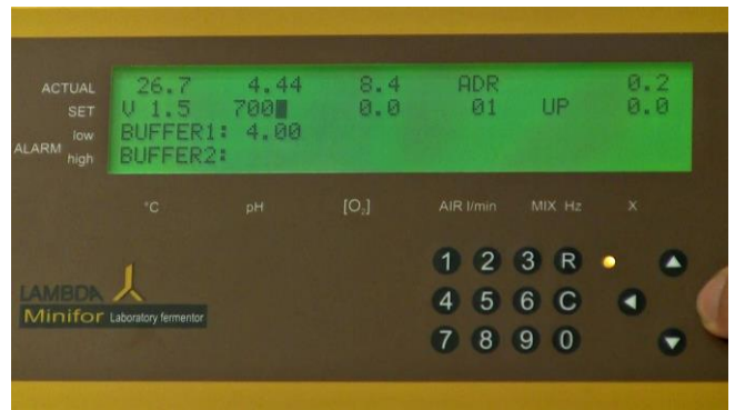
Figure 5.2—10 Start the calibration of the second gauging solution, by entering the next pH value and then press the right arrow key ">" to SET the needed pH value. For example: Enter 700 for pH 7.
