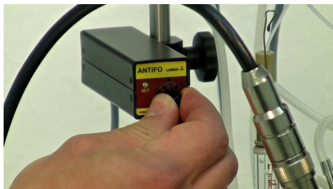
Figure 5.6—2 Rotate the ANTIFO knob clockwise gently to find a point where the green LED turns to yellow as shown.
