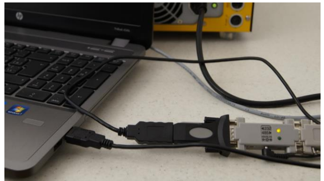
Figure 6.4—6 The PC connection cable along with the RS converter is connected to the PC with the help of the USB connector.
