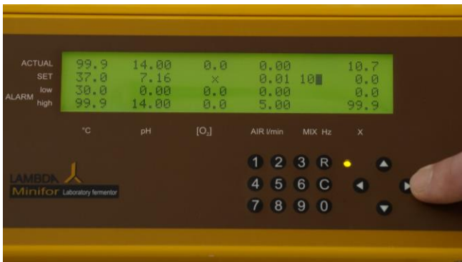
Figure 4.3—5 Move the cursor using the navigation key and place it on the MIX Hz column. Set the desired frequency of agitation using the number keys and press the right arrow for saving the entered value.
