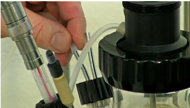
Figure 3.11-5 Slip the tubing for cooling liquid inlet over one of the steep tubes of the cooling loop as shown.
