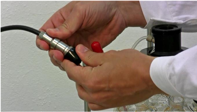
Figure 3.15—5 Take the pH probe connector from the base unit of the MINIFOR Bioreactor. (Black cable from the base unit). Remove the black protection cap on the sensor (top part) of the cable.
