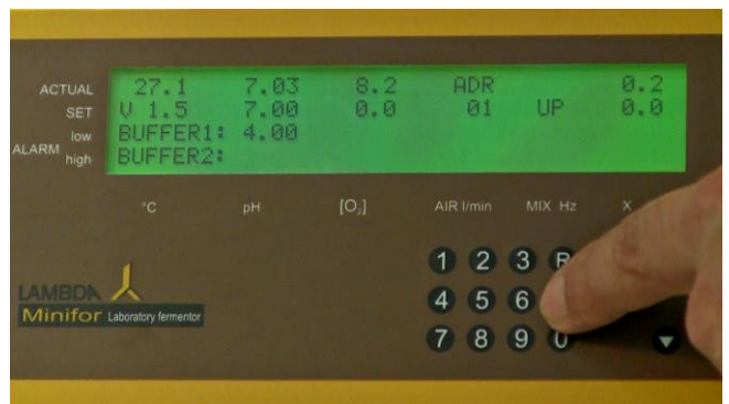
Figure 5.2—14 Once the value becomes stable, press the calibration key “C”. The calibrated value will be saved and displayed as BUFFER 2 pH value.
