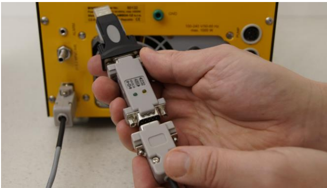
Figure 6.4—3 Connect the RS-485 to RS-232 converter to the other end of the PC connection cable.
