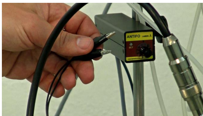
Figure 3.15—27 The two crocodile clips of the ANTIFO need to be connected with the cannulas from the quadruple sampling port for the detection of the foam level in the working vessel.
