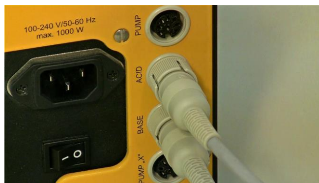
Figure 3.16—17 Connect the acid Peristaltic pump remote cable into the 'ACID' socket on the MINIFOR base control unit.
