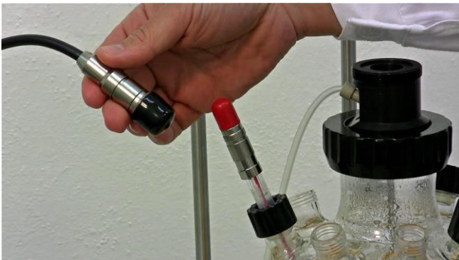
Figure 3.8-9 Take the pH probe connector from the base control unit of the MINIFOR Bioreactor. (Black cable from the base unit)
