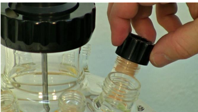
Figure 3.7-7 Place the black screw cap loosely on to the stopper and washer.
