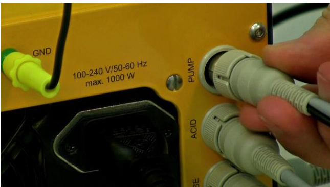
Figure 3.15—33 Connect the grey colour ANTIFO cable (8 poles) to the "PUMP" socket present on the rear of the MINIFOR base control unit.
