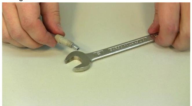
Figure 3.5-10 Picture shows the prepared PEEK double-seal tubing connector.
