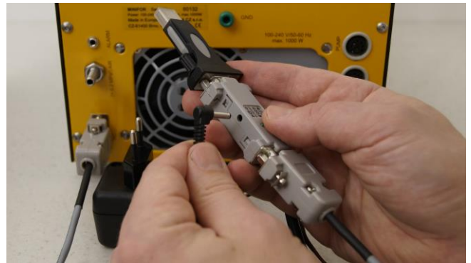
Figure 6.4—4 Plug in the power supply for the RS-485 to RS-232 converter.
