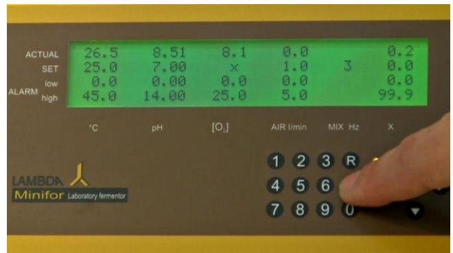
Figure 4.1—2 "C" - Calibration key is pressed to change the stand-by mode to calibration mode.
