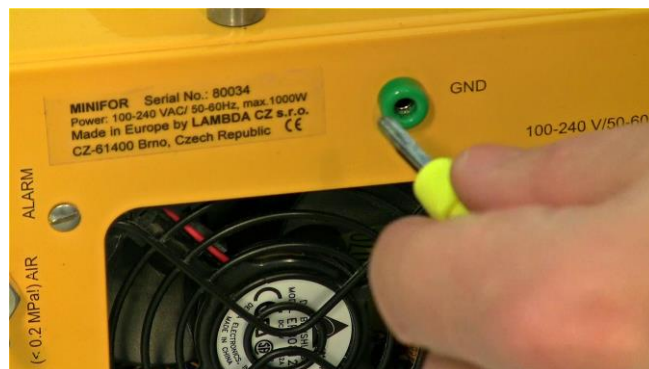
Figure 3.15—35 Connect the black cable with green connector to "GND" at the rear of the MINIFOR base unit for grounding (or earthing).
