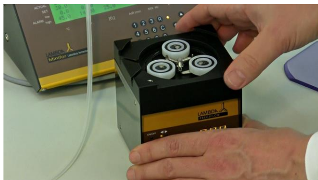
Figure 3.16—2 Remove the transparent PVC head cover. The speed of rotation has to be increased using the “▲▲▲” arrows present below the LED display.
