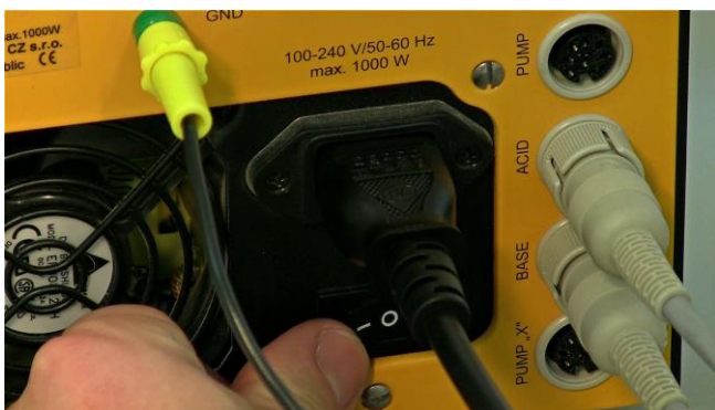
Figure 3.15—44 Once the connections and installations are done, switch on the MINIFOR using the power switch present below the power input. (Power Switch: I = On; O = Off)
