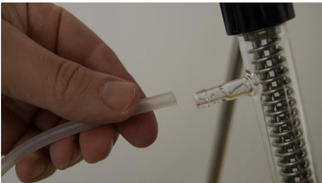
Figure 3.12-14 Connect a tubing to the outgas condenser cylinder and lead the tubing to a glass vessel or flask.
