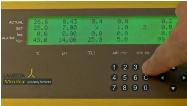
Figure 5.3—14 Press the regulation key "R" to change the calibration mode to standby mode. Since the calibration is just complete, pO 2 probe will be still merged in the O 2 -saturated medium / liquid.
