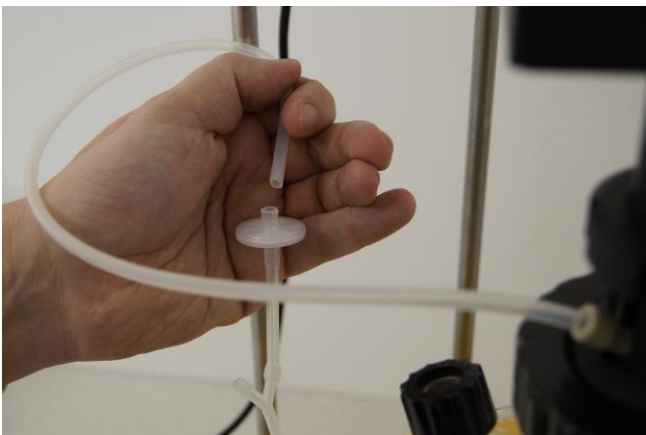
Figure 3.6-11 Connect the tubing with the filter from Y-piece to the sparger.
