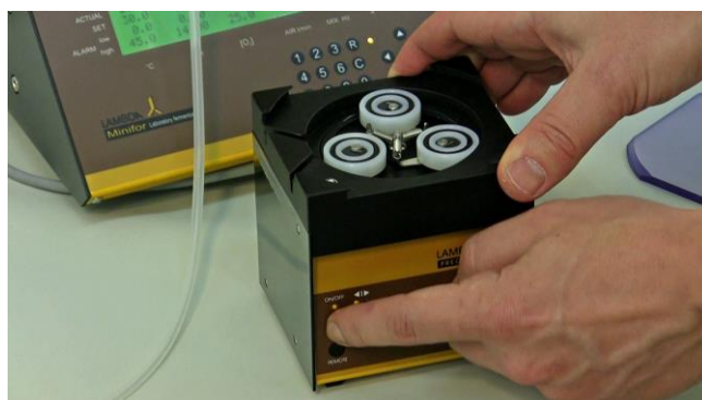
Figure 3.16—4 Press the ON/OFF button and select the sense of rotation of the pump by pressing the button ◀▶
