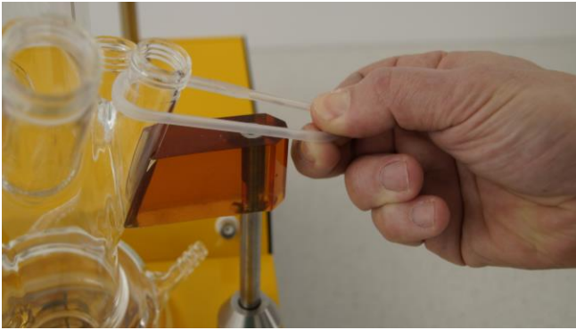
Figure 3.4-17 Place the elastic silicone ring on the distinct side arms of the pH and pO 2 probe.
