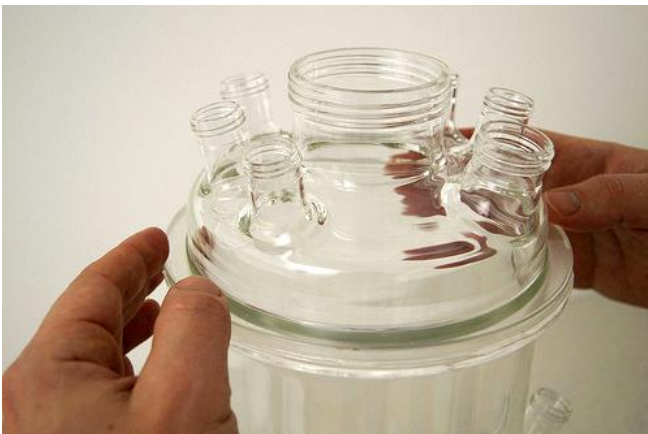
Figure 3.4-27 Place the upper part onto the lower vessel part. The paste fills any cavity between the joining surfaces and is completely gas tight and also does not generate any stress in the glass.
