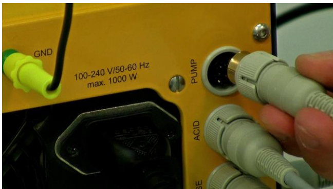
Figure 3.11-15 Connection for the Peltier cooling device: on the rear of the MINIFOR.
