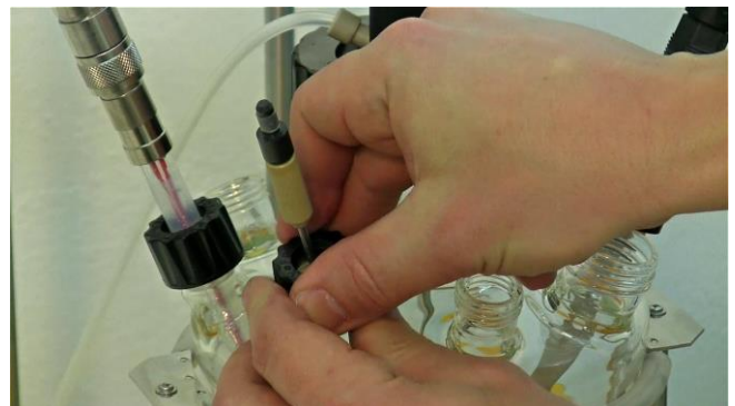
Figure 7.1—2 Check whether the over-pressure valve has been inserted in the vessel.
