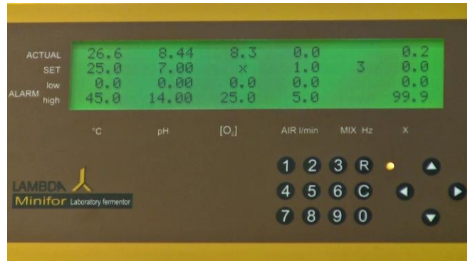
Figure 5.3—15 The measurement of the O 2 saturated medium / liquid will be displayed in the ACTUAL Value of the parameter [O 2 ].
