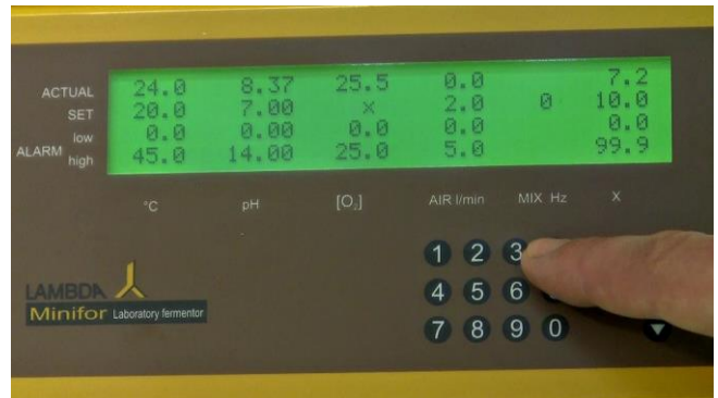
Figure 5.5—19 Press the regulation key "R" to exit the calibration mode.
