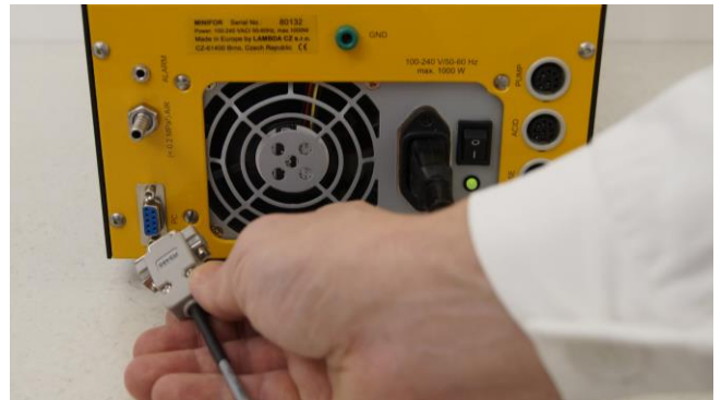
Figure 3.15—39 Connect the PC connection cable to the DB 9 connector at the rear of the base control unit.
