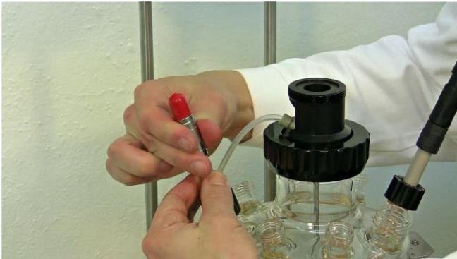
Figure 3.8-7 Carefully insert the pH probe on the pre-prepared port with the stopper, washer and black screw cap.
