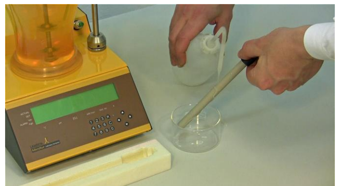
Figure 3.7-8 Moisten the pO 2 (DO) probe with de-ionized water to ease insertion of probe.
