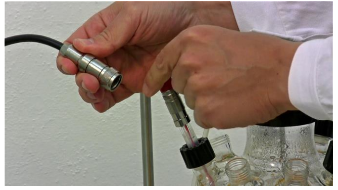
Figure 3.15—6 Remove the protective cap from the pH probe (red cap)
