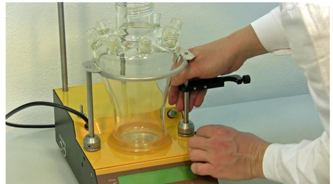
Figure 3.4-12 Tighten the slots also on the other side so that it's secure. (N.B. If you will need to use the sterile sample device you can attach the holder to e.g. the right-hand support)
