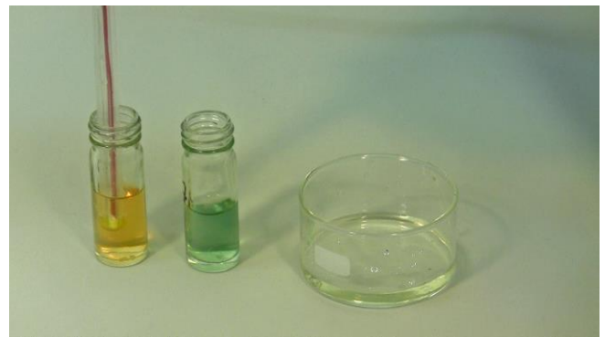
Figure 5.2—6 Dip the probe into the gauging solution (pH 4 buffer solution) and stir gently while the pH is being measured.
