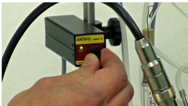
Figure 5.6—1 Once the connections are made, the ANTIFO LED will be illuminated as green.
