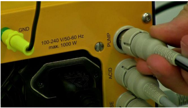
Figure 3.15—9 Peltier cooling finger can be directly connected on the “PUMP” socket present at the rear of the MINIFOR base control unit.
