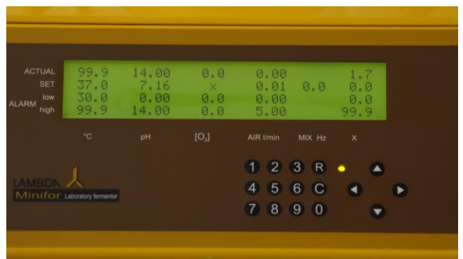
Figure 3.15—45 When switched on, the MINIFOR starts with a beep sound and yellow LED display on the control panel. This represents the Stand-by mode of the MINIFOR fermentor-bioreactor.
