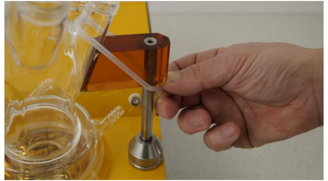
Figure 3.4-18 Pull the elastic silicone ring and affix the side arms of the vessel with the lateral reaction holder.
