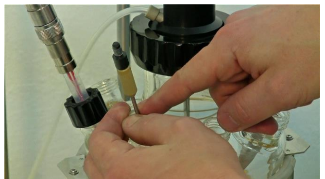
Figure 3.9-4 Insert the stopper with the pressure limiting security valve into the port. (Probably the Pressure limiting security valve can be placed beside the pH probe port on either side)
