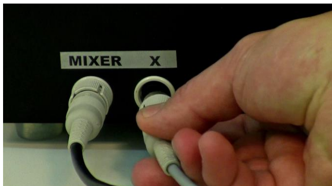
Figure 3.15—25 Connect the weighing module connection cable in the “X” socket beside the “MIXER” on the left side of the MINIFOR base control unit.
