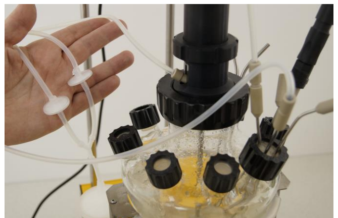
Figure 3.6-14 Secure the tubing to the sparger with a lock when surface sparging is used.
