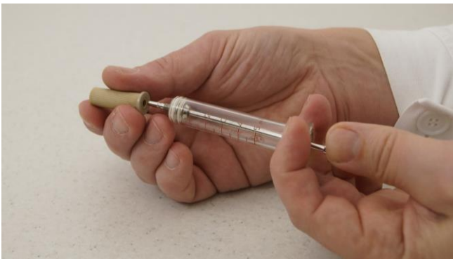
Figure 3.14—7 Push the plunger completely along the barrel of the syringe to mechanically fix the metal outlet tip. Insert the PEEK adapter body on the threaded syringe tip and tighten it securely by screwing.
