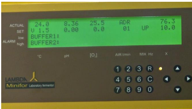
Figure 5.5—5 Entered 100 will appear as 10.0 in the SET display after pressing the right arrow key.
