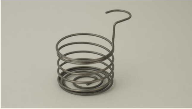
Figure 7.2—1 Storage bottle holders during sterilization.
