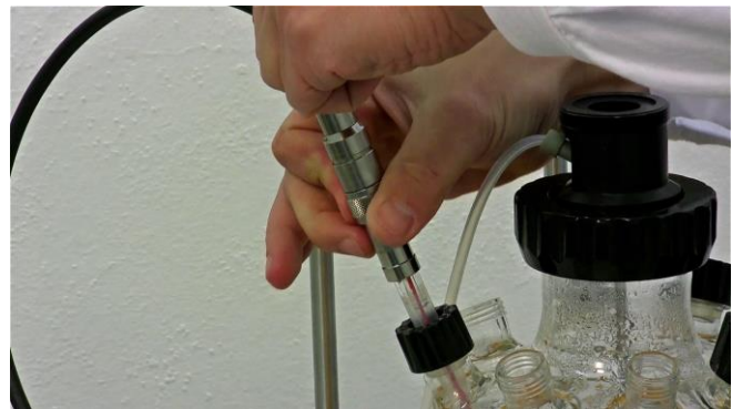
Figure 3.15—8 After locking the pH probe and connector cable; tighten the connection by screwing the threaded lock on the connector cable by rotating as shown.
