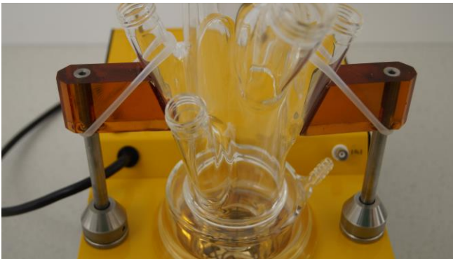
Figure 3.4-19 The reaction vessel mounted on the base unit and made intact with the help of the lateral holder and elastic silicone ring.
