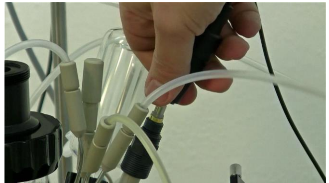
Figure 7.1—6 Disconnect the pO 2 probe connector cable from the pO 2 probe.
