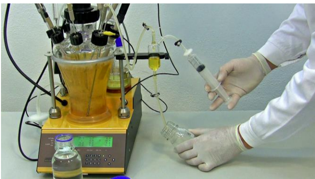
Figure 8.2—7 Use a beaker / bottle to collect the flushed waste sample. Push the syringe plunger to pass the air drawn into the sampling device and thus making the flow of the flushing liquid from the sampling device into the wastage bottle.
