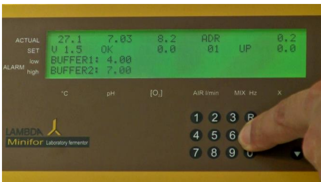
Figure 5.2—15 OK message will be displayed, if the calibration is done correctly.
