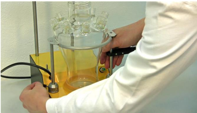
Figure 3.4-11 While supporting the reaction vessel holder with one hand, tighten around the slots of the reaction vessel holder with the given key.
