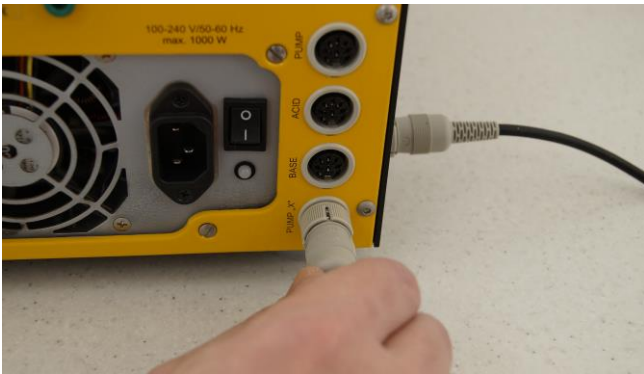
Figure 3.13—8 Connect the corresponding pump to the “PUMP X” *) socket on the rear of fermenter-bioreactor MINIFOR.
