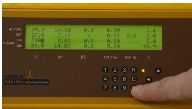
Figure 4.3—3 Move the cursor on the field of temperature minimum (ALARM LOW). Enter the desired value. If the temperature falls below this value, an alarm is activated and an asterisk is displayed on the left of the corresponding value.
