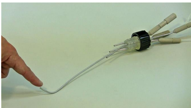
Figure 3.15—36 The grounding (or earthing) cable has to be connected with the longest cannula in the quadruple sampling port.
