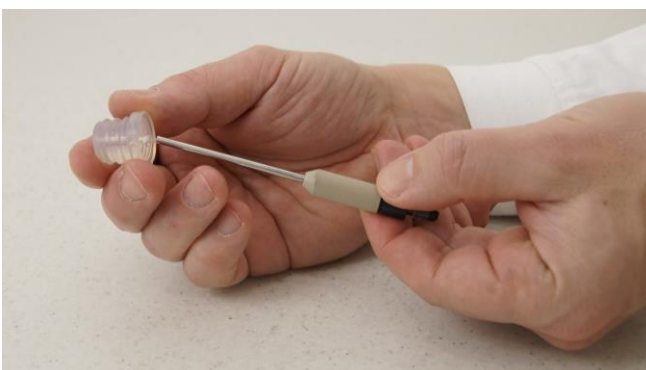
Figure 3.9-3 Insert the assembled over pressure limiting security valve to the rubber stopper.
