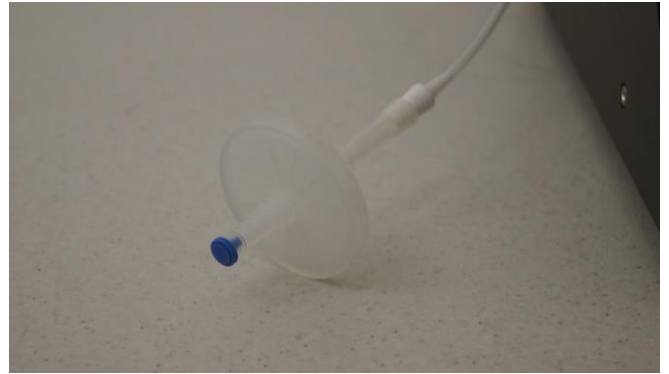
Figure 3.6-4 Picture shows the connection of the air-inlet filter with the tubing from the head of the agitation unit using the tubing connector.
