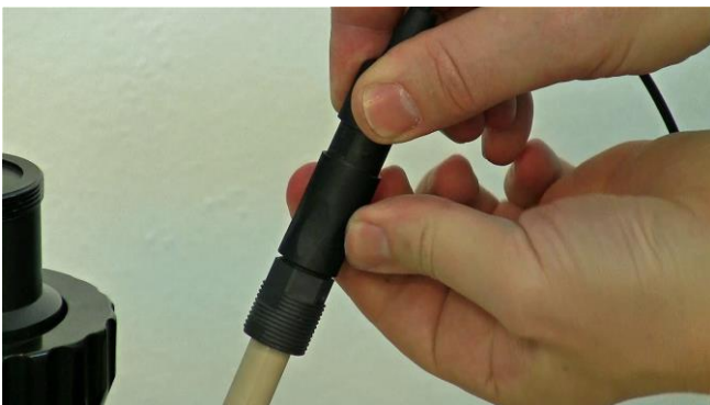
Figure 3.7-13 After fixing the pO 2 (DO) probe and connector exactly in locking position, push down the sleeve of the pO 2 (DO) probe connector and secure it sufficiently with screw fitting.
