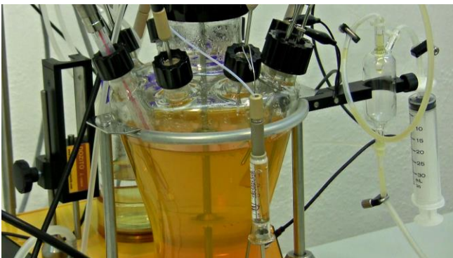
Figure 3.14—16 Hook the Syringe, with the help of the holder fitted in the PEEK head, in the one of the needle/cannulas inserted in the port.
