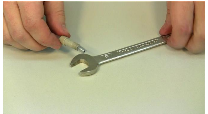
Figure 3.10-10 Picture shows the prepared PEEK double-seal tubing connector.
