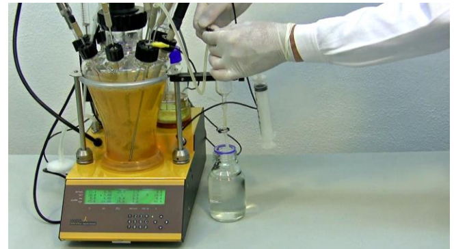
Figure 8.2—2 Open the clamp on the sampling inlet (i.e. Between the MINIFOR and the sampling device)
