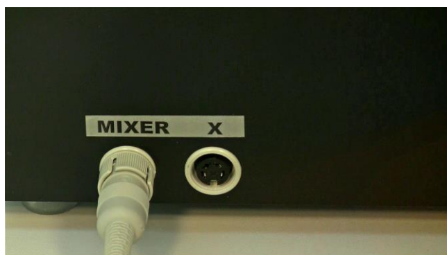
Figure 3.15—4 Connect the agitation unit cable to the "MIXER" socket present at the left side of the MINIFOR Base Unit.
