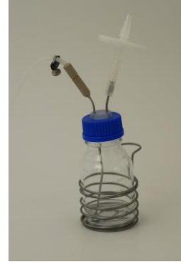
Figure 7.2—2 Clap the tubing and check that the filter is not clogged. Place the bottles in the sterilization storage bottle holder.
