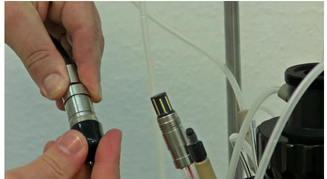
Figure 7.1—8 Protect the female cable connector using a cap against contamination.
