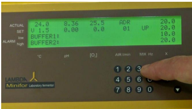
Figure 5.5—13 Press the regulation key "R" to exit the calibration mode.
