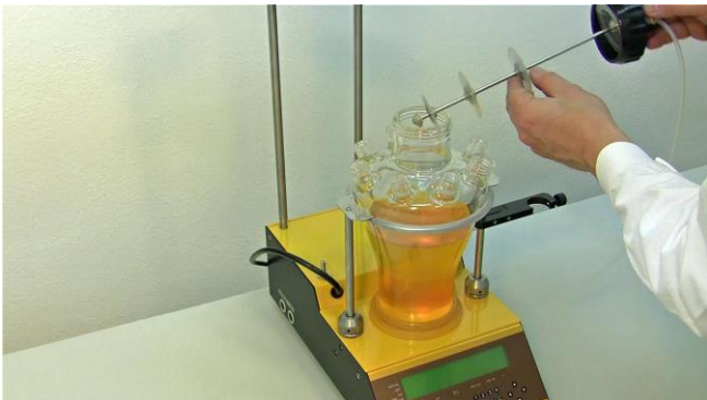
Figure 3.5-25 Place the agitation unit with the fish tails discs and microsparger into the vessel and fix the central screw cap on the reaction vessel.
