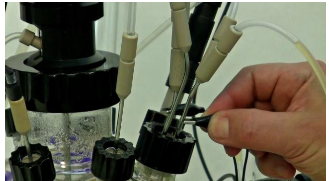
Figure 3.14—6 Adjust the tip position of the “foam”-needle just above the medium level, where the foam should be controlled. Connect the second crocodile clip to the selected short needle.
