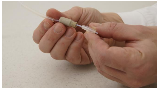
Figure 3.14—8 Insert the double conical silicone insert with the PTFE tubing into the double seal PEEK fitting part through a small segment of silicone tubing, to avoid bending of PTFE tubing.
