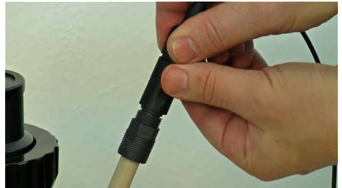
Figure 3.7-12 Place and adjust the pO 2 (DO) probe connector by rotating to find the position for exact locking of grooves with the pO 2 (DO) probe.
