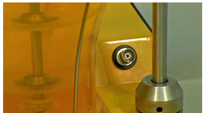
Figure 5.3—9 DO probe should only be removed for not more than 1 minute as it lead to lose the polarization. If it is any longer than 1 minute, this will result in inaccurate readings.
