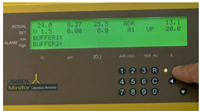
Figure 5.5—17 Use the up arrow navigation key to change from DOWN to UP.
