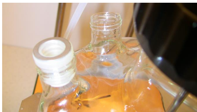
Figure 3.8-4 Make sure that the washer is placed on the white open stopper.
