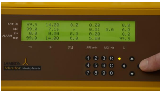
Figure 4.3—1 Move the cursor by using arrows on the field for the temperature setting (SET °C, second row, first column).
