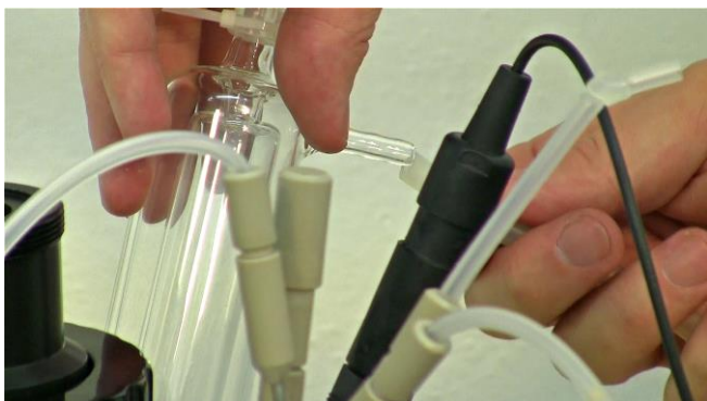
Figure 3.12-5 Connect the cooling water to the outgas condenser. (Lower arm = inlet, Upper arm = outlet for cooling water).
