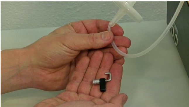
Figure 3.6-7 The safety lock is provided for the air input. This protects the air-input filter for liquids entering the air-output / air-input line).
