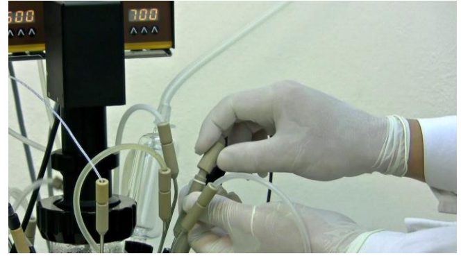
Figure 8.2—6 Replace the septum protection cap securely.
