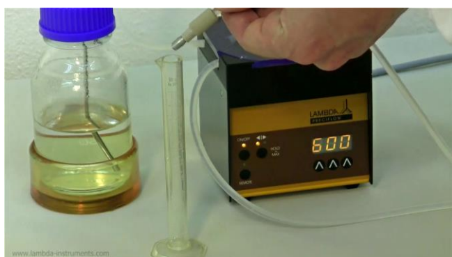
Figure 5.4—3 Collect the liquid in the measuring cylinder for about 60 seconds.
