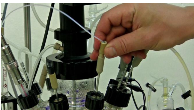
Figure 3.14—27 Insert the PEEK connector with the PTFE Antifoam tubing into the cannula as shown and secure the tubing firmly to the cannula.
