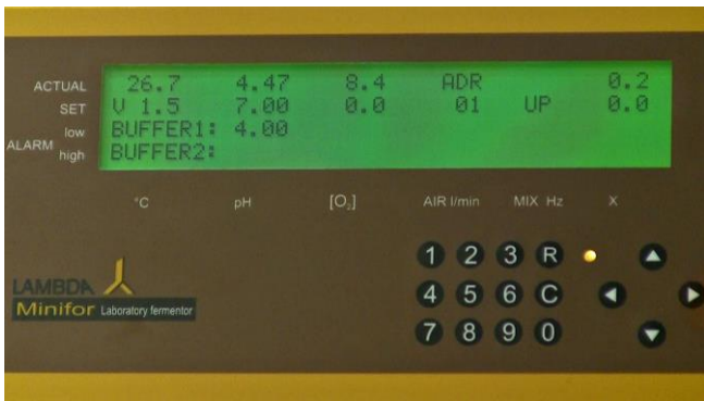
Figure 5.2—11 After pressing the right arrow key “>”, the value entered (700) will be SET as pH 7.00.
