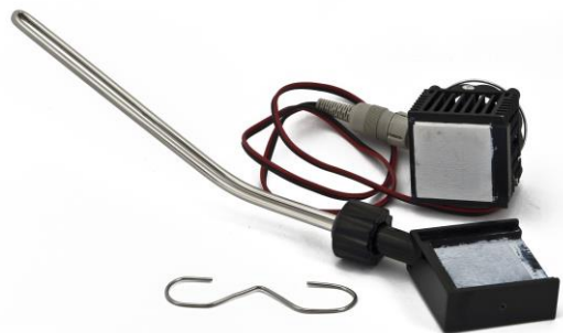
Figure 3.11-8 Detached parts of the Peltier cooling finger.
