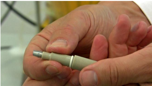
Figure 3.10-15 Fix the septum protection cap on the threaded side of the white septum O-ring.
