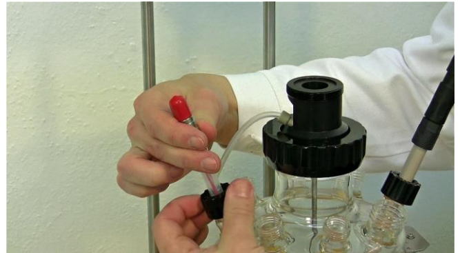
Figure 3.8-8 Tightly secure the black screw cap, after insertion of the pH probe.
