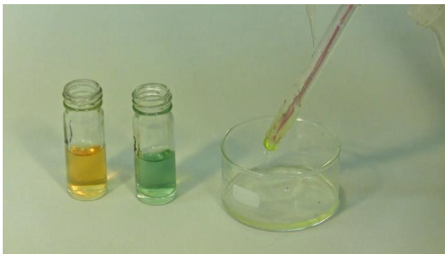
Figure 5.2—21 Rinse the probe again and dry it with the blotting paper.
