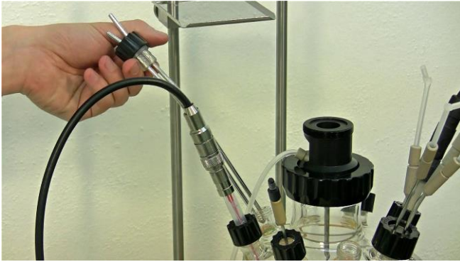
Figure 3.11-3 Place the cooling loop in the desired neck at the back of the vessel to leave it undisturbed.
