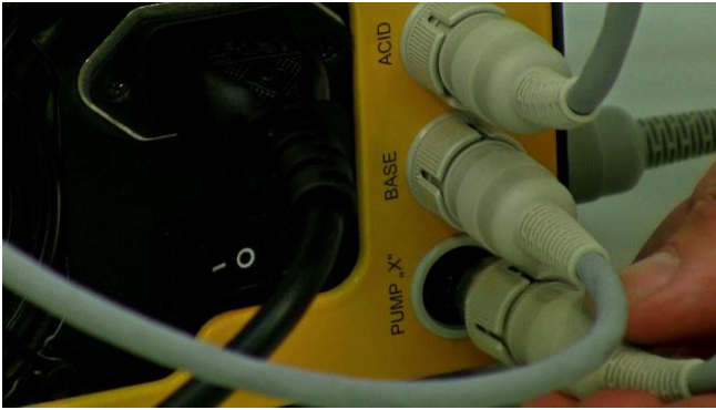
Figure 3.16—18 Feed or the Harvest pump of the weighing module should be connected to the PUMP 'X' socket.
