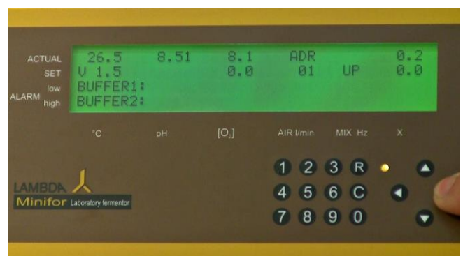
Figure 5.3—4 Check the ACTUAL value of the temperature (this should be the desired temperature for the run). Refer the corresponding Oxygen saturation value for the temperature in the table 5.3.4 Oxygen saturation in water. [e.g. oxygen saturation in water at 26.5°C = 8.0 mg O_2/l ]
