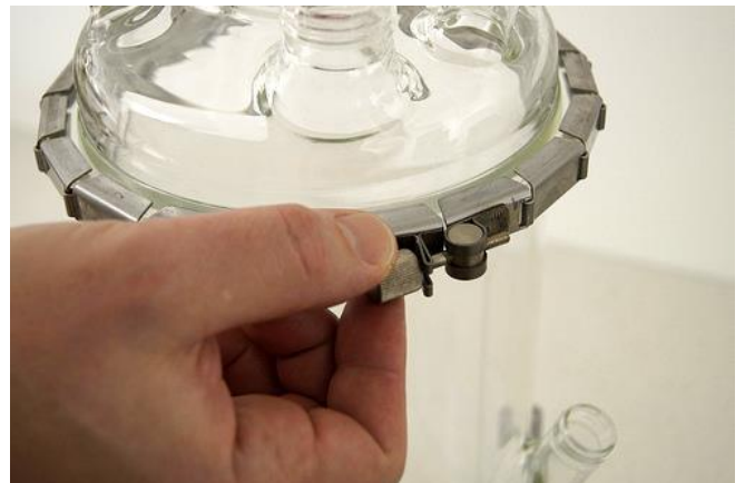
Figure 3.4-28 Fix them together with the segmented vessel closing belt. The mixture will cure either during staying at room temperature in several hours or within minutes in the autoclave during sterilization.
