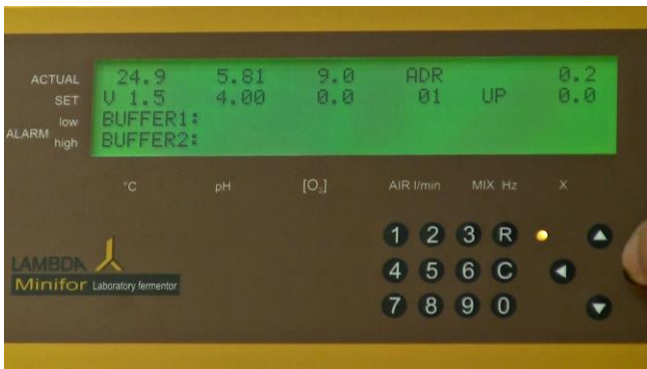
Figure 4.1—6 Once the cursor is activated after the long press of “C” key, pressing the arrows will move the cursor to the corresponding direction.
