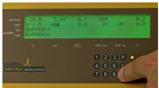
Figure 4.1—8 Changing the value of the selected parameter using number keys.
