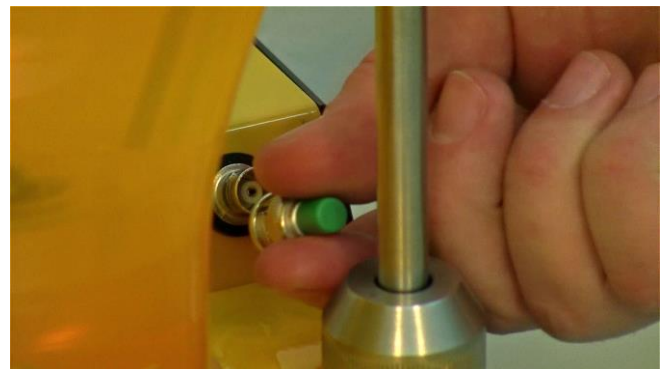
Figure 3.7-14 Remove the protection cap by pressing and unlock by rotating from the pO 2 (DO) probe socket on the base control unit.
