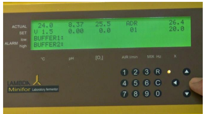
Figure 5.5—15 Press the right arrow navigation key (>) to select the SET value "UP" in the column before the parameter "X".
