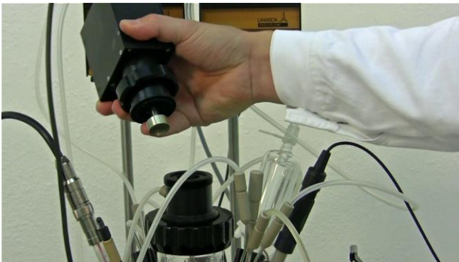
Figure 7.1—5 Remove the agitator from the agitation unit. Carefully tilt the agitator back and forth for easy removal.
