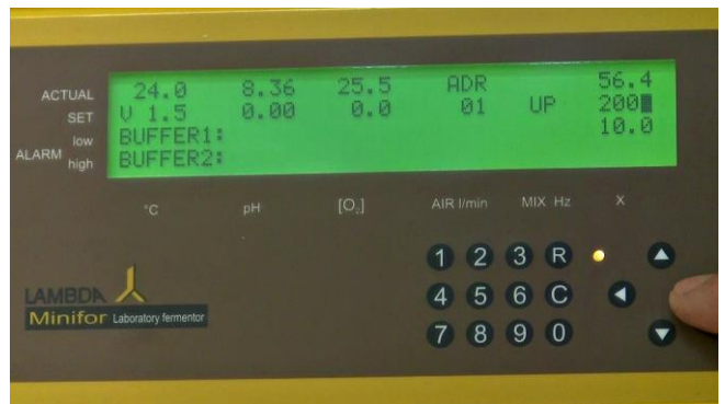
Figure 5.5—10 Enter the final value to be detected and controlled by the scale module. For example: enter 200 and press the right arrow key (>) to save the value.
