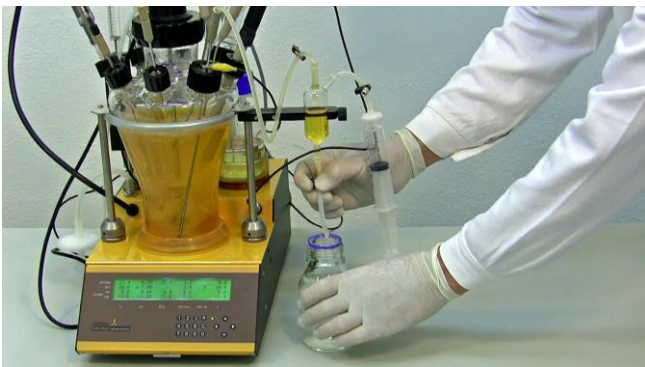
Figure 8.2—5 Remove the 70% Ethanol beaker / bottle into which the outlet tubing is dipped.
