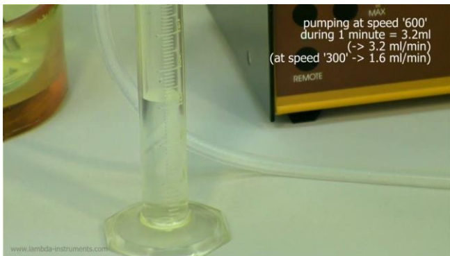
Figure 5.4—5 Measure the volume of liquid collected in a minute. At the speed of 600, 3.2 ml/minute has been collected. Calculate the flow rate for other speed range using this value.
