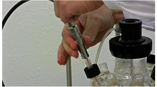
Figure 3.8-12 After locking the grooves of the pH probe and connector cable, tighten the connection by screwing the threaded lock on the connector cable by rotating as shown.
