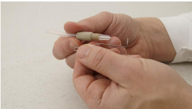
Figure 3.14—9 Insert the holder for autoclaving to the threaded neck of the double seal PEEK fitting part.
