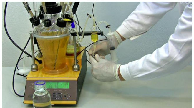
Figure 8.2—6 Open the clamp on the outlet tubing.
