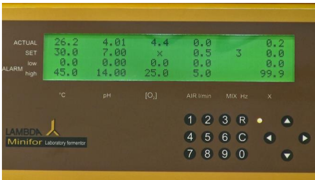
Figure 5.2—23 The ACTUAL value of the parameter pH on the display should be 4.00 (It can range between 3.96 – 4.04)
