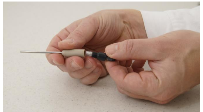
Figure 3.9-2 Insert the other end with the stainless steel cannula with LAMBDA PEEK connector.
