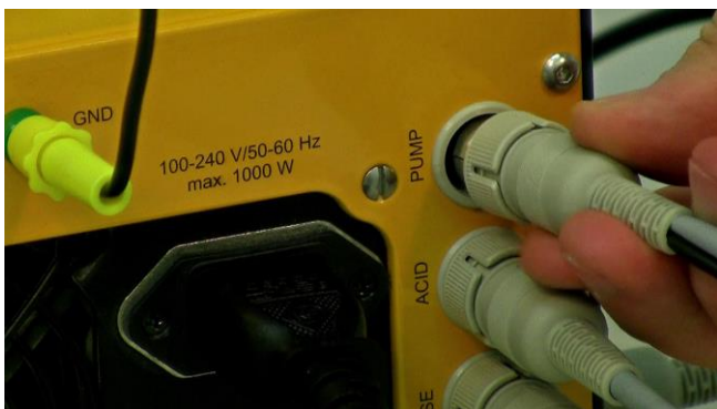
Figure 3.14—25 Connect the ANTIFO cable (8 poles) to the “pump” socket present on the rear of the MINIFOR base control unit.
