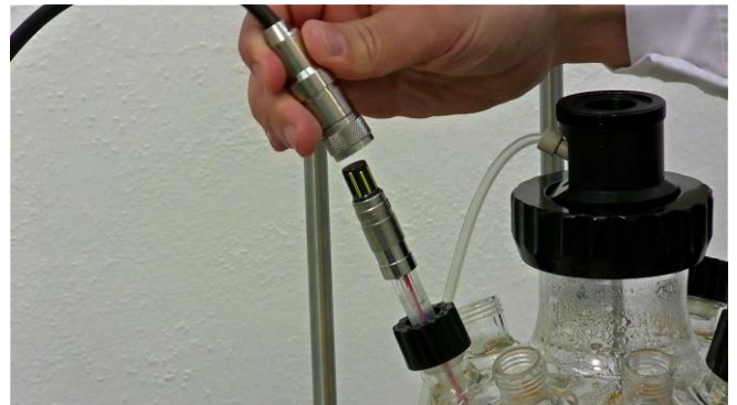
Figure 3.8-10 Remove the black protection cap on the sensor (top part) of the cable and red protective cap from the pH probe.
