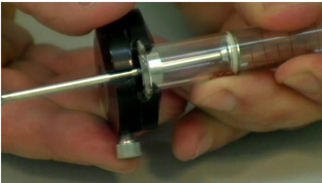
Figure 3.14—14 Rotate the holder with firmly holding the syringe, in order to fit the syringe securely in position.
