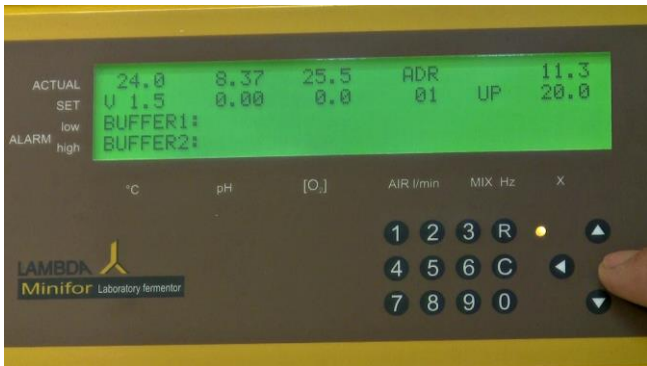
Figure 5.5—18 Press the right arrow navigation key to save the value, once the regulation of pump is selected.
