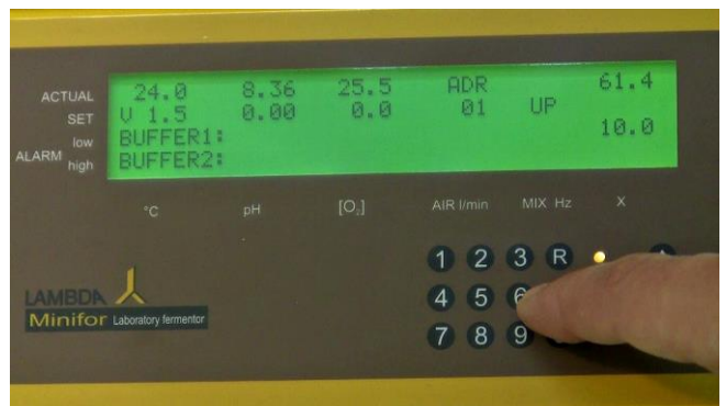
Figure 5.5—8 Once calibrated, the initial value will appear as BUFFER 1 value of the parameter “X”.
