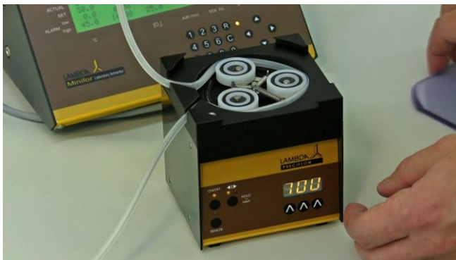
Figure 3.16—7 Press the tubing into the front slot to secure it.
