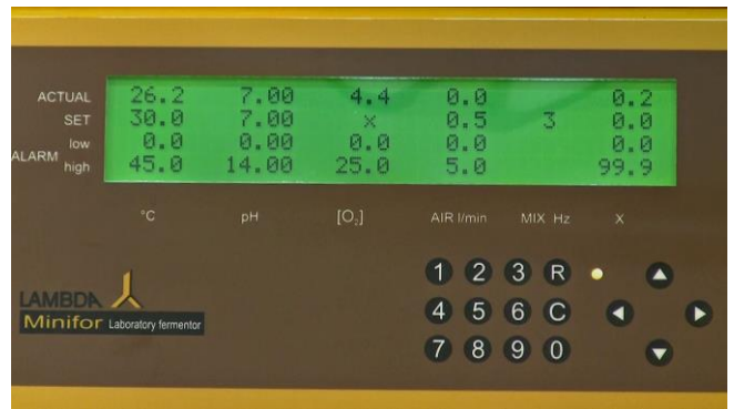
Figure 5.2—20 The ACTUAL value of the parameter pH should be 7.00 (It can range between 6.95 – 7.04)
