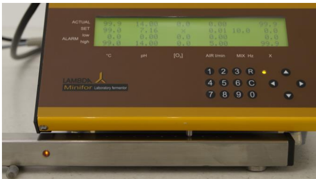
Figure 3.13—5 If the weight of the filled vessel exceeds the measurement range, a roof sign “^” will appear in the measured (actual) weight value [Refer Actual value of the parameter “X” in the display] and a red LED light will be displayed in the weighing module.
