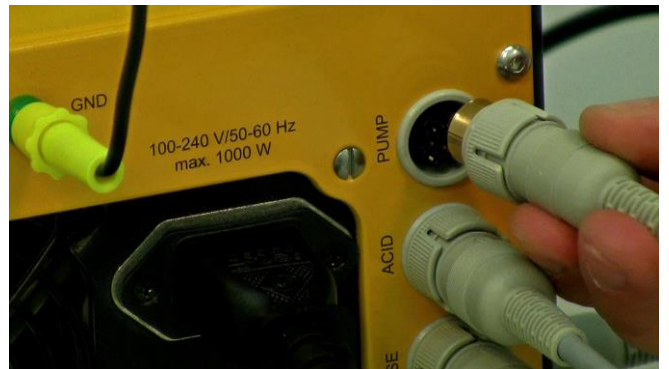
Figure 3.12-15 Connection for the Peltier cooling device: on the rear of the MINIFOR.
