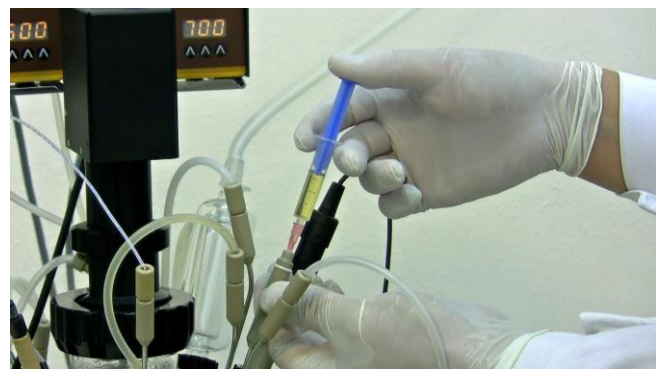
Figure 8.2—4 Inject the inoculum / inoculant into the liquid medium.
