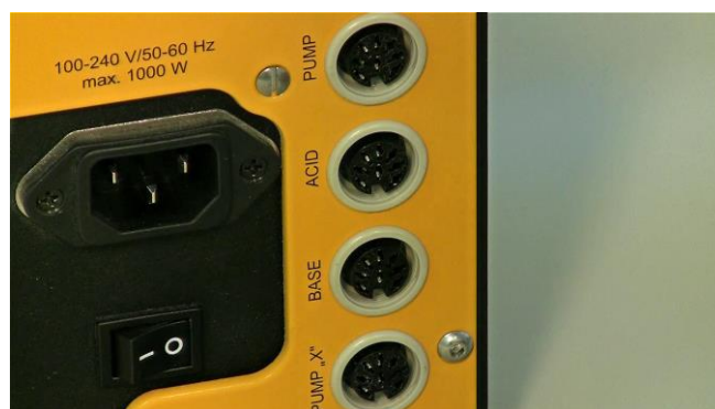
Figure 3.16—15 Pumps has to be connected into the respective sockets at the rear of the MINIFOR base control unit.
