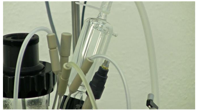
Figure 7.1—12 Clamp all the tubings and air input line except the air output line with the out gas condenser and output filter.
