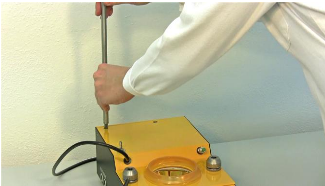
Figure 3.3-1 As a first step, insert the support rods in the present basic control unit as shown. Rotate it clockwise for fixing.
