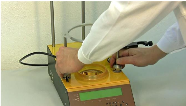
Figure 3.4-7 Deeply insert the reaction vessel holder into the desired slots.
