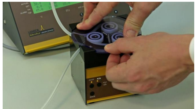
Figure 3.16—8 Replace the transparent PVC head cover and twist it gently to secure it.
