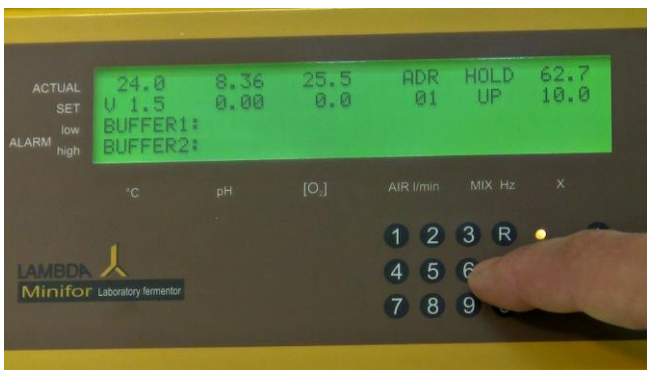
Figure 5.5—7 Observe the actual value of the measured weight. When the reading becomes stable, wait until the message “HOLD” appears. And then press the calibration key “C” to calibrate the initial value.
