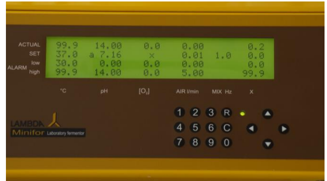
Figure 4.2—2 Regulation / Operation mode - The regulation is activated by pressing key "R" and the LED turns to green. The display shows the measurement of all the parameters.
