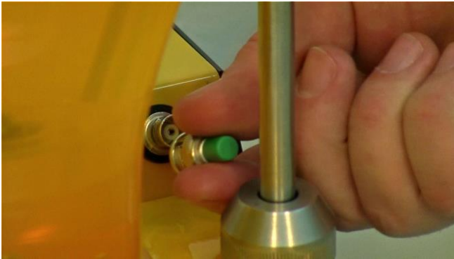
Figure 3.15—19 Remove the protection cap by pressing and unlock by rotating from the pO 2 (DO) probe socket on the base control unit.
