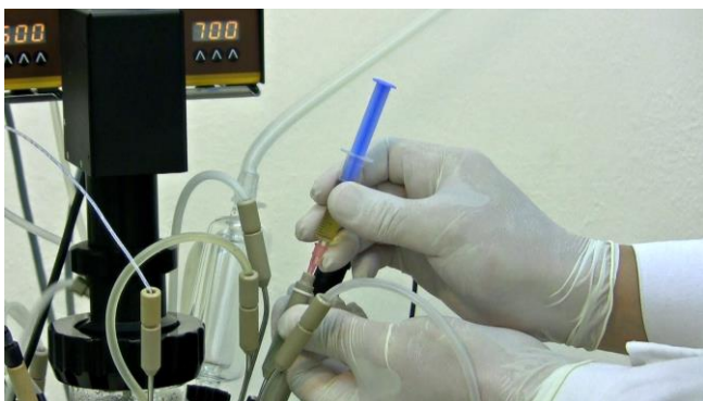
Figure 8.2—3 Insert syringe loaded with the inoculum / inoculum along with the syringe needle into the septum adaptor body.
