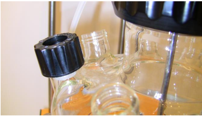
Figure 3.8-5 Place the black screw cap loosely on the white open stopper and washer.
