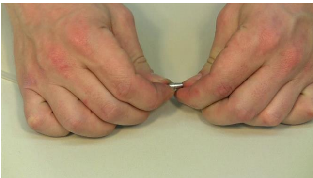
Figure 3.5-7 Insert the double-seal conical insert into the tubing which is freely flowing on the other side of the PEEK fitting.
