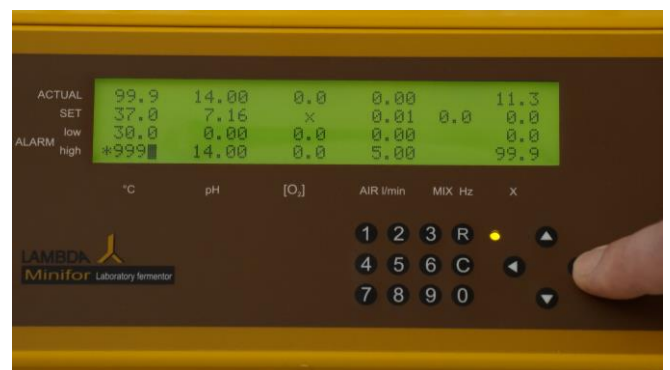
Figure 4.3—7 Alarm can be deactivated by changing the alarm high value and by taking needed precautions to maintain the temperature.
