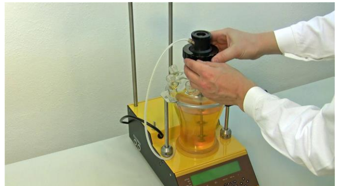
Figure 3.5-26 Ensure that the large central screw cap for head fixing is securely tightened to the rim of the reaction vessel. See that the mobile PEEK cock tubing for air input is positioned as in the figure.
