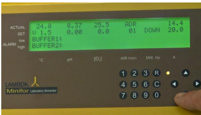
Figure 5.5—16 Use the down navigation key to change to DOWN option.
