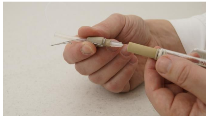
Figure 3.14—10 Insert the prepared double seal PEEK fitting part with conical silicone insert and PTFE tubing to the PEEK adapter connected with the syringe.
