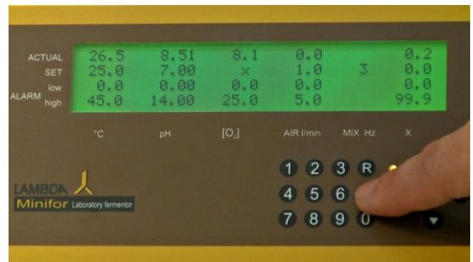
Figure 5.3—2 Make sure that the agitation value entered as SET value. Press the calibration key "C". (Please note that the agitation of the medium take place even in the calibration mode).
