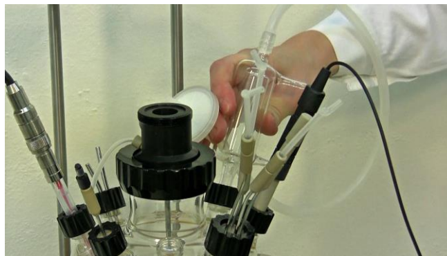
Figure 3.12-3 Insert the outgas condenser into the port with the open stopper, washer and black screw cap. Select a port that will not be disturbed during the work.
