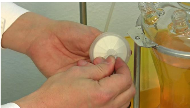
Figure 3.6-5 Connect a small piece of tubing (cut as desired) to the shown free end of the air-input filter.
