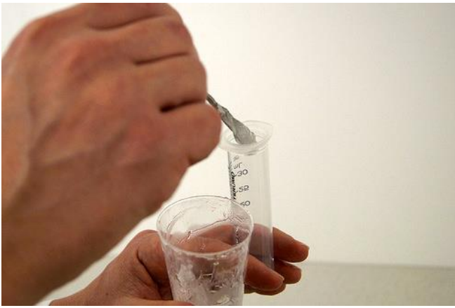
Figure 3.4-23 Transfer the prepared liquid O-ring into a syringe for an easy application of the mixture in the vessel.
