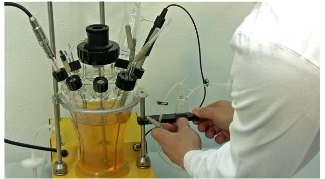
Figure 3.10-24 Place the sterile sampling device on the sterile sampling device holder (Refer 3.4 Setting up of fermentation Vessel) and tighten it with the side-screw.
