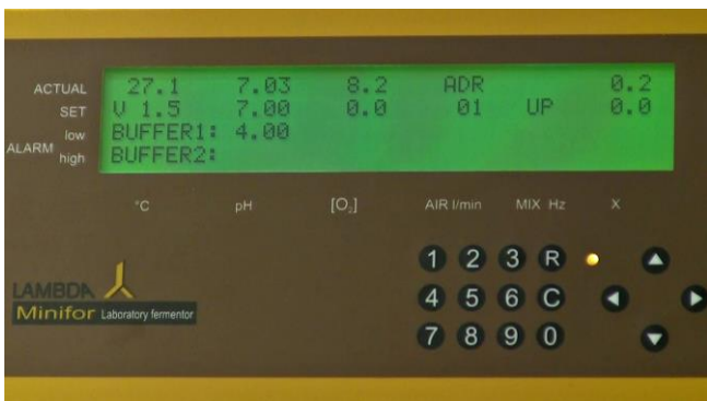
Figure 5.2—13 Wait until the ACTUAL value if the gauging solution becomes stable.
