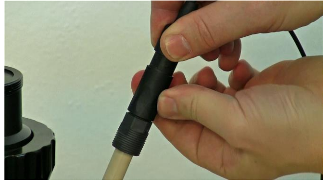
Figure 3.15—18 After fixing the pO 2 (DO) probe and connector exactly in locking position, push down the sleeve of the pO 2 (DO) probe connector and secure it sufficiently with screw fitting.
