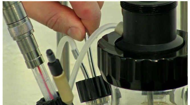
Figure 3.11-6 Slip the tubing for the cooling liquid outlet over the other tube of the cooling loop to allow the flow of cooling liquid throughout the cooling loop.
