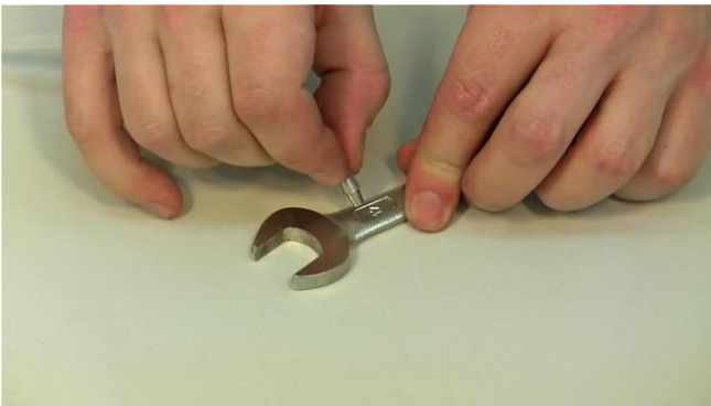
Figure 3.10-9 Take a spanner and the double seal conical insert with the tubing. Press the conical insert with the tubing against the spanner to make it inserted totally into the tubing.
