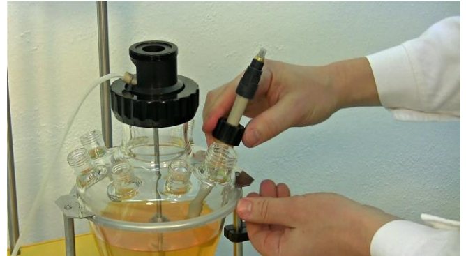
Figure 3.7-10 Tightly secure the black screw cap placed on the top of the coloured stopper.
