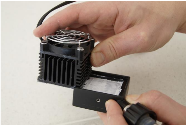
Figure 3.12-6 Detach the Peltier cooling element with control electronics and fan from the condensing finger as shown while preparing for sterilization.
