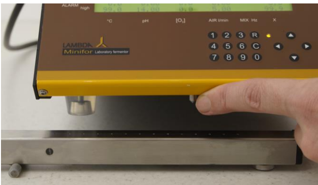
Figure 3.13—1 The steel hard tip can be found under the front part of the MINIFOR unit (miniature scale module). Place the weighing module under the front part of the MINIFOR.
