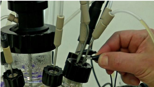
Figure 3.15—31 Connect the second crocodile clip to the selected short needle.
