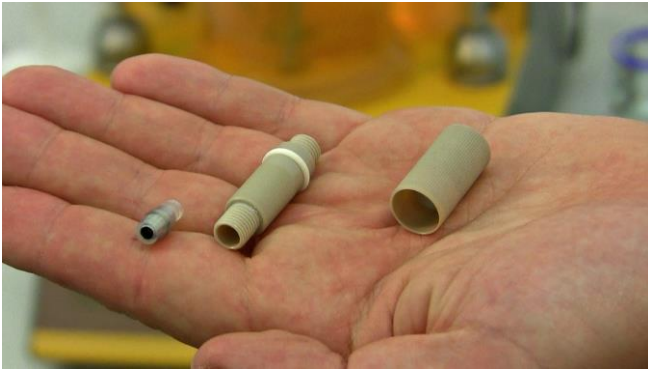
Figure 3.10-11 Parts need to be connected together to form the inoculation device. From left to right; 1. The tubular septum containing the double seal conical insert for tubing inside; 2. The septum adaptor body with a white septum O-ring for septum adaptor body; 3. The septum protection cap containing the sealing disc.
