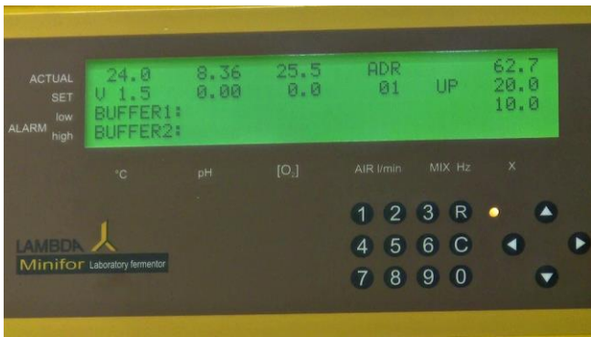
Figure 5.5—11 The entered 200 will appear as 20.0 in the SET value after pressing the right arrow key (>).
