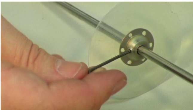
Figure 3.5-21 Fasten the fish tails on the sparger pipe with one of the keys supplied. (E.g. the screw piece can be facing down for all fish tails)
