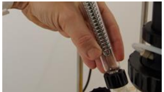
Figure 3.12-13 Peltier outgas condenser can be placed in the same place as that of glass condenser. Secure it tightly with care using the black screw cap, since the head of the Peltier outgas condenser may be slightly heavier, while fastening the screw cap.
