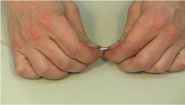
Figure 3.10-7 Insert the double-seal conical insert into the tubing which is freely flowing on the other side of the PEEK fitting.
