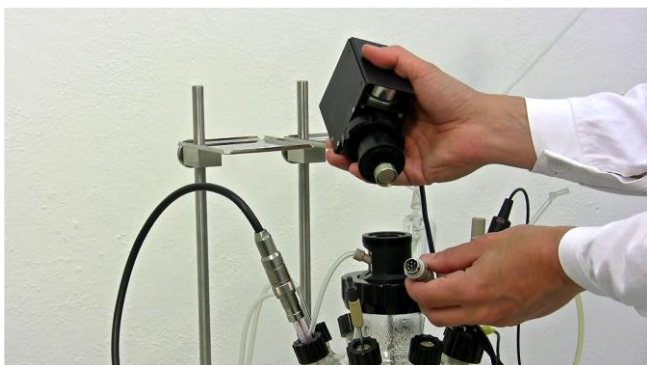
Figure 3.15—1 Take the vibromixer with the cable and fittings.
