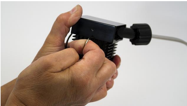
Figure 3.11-13 Locking clamp has to be pulled firmly through the Peltier cooling element with control electronics and fan, to ensure good heat transfer to the cooling loop.
