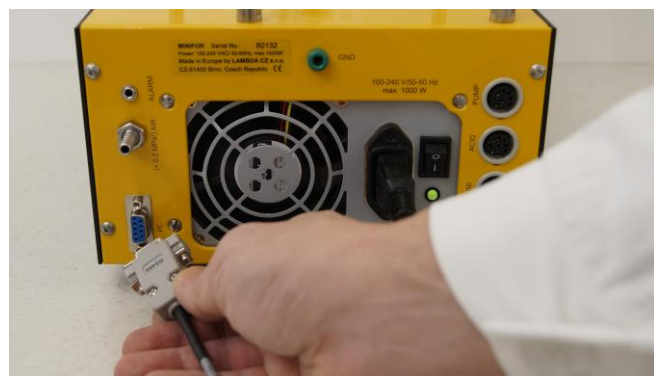
Figure 6.4—2 Connect the PC connection cable to the DB 9 connector at the rear of the base control unit.
