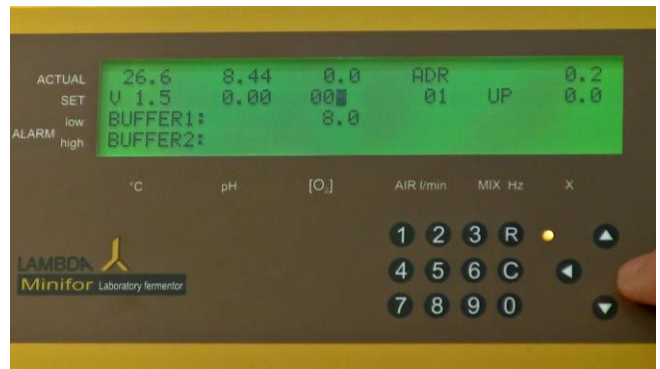
Figure 5.3—11 Enter the SET [O 2 ] value 00 using the number keys and press the right arrow key to save the value. The value will be displayed as 0.0 in the SET value.
