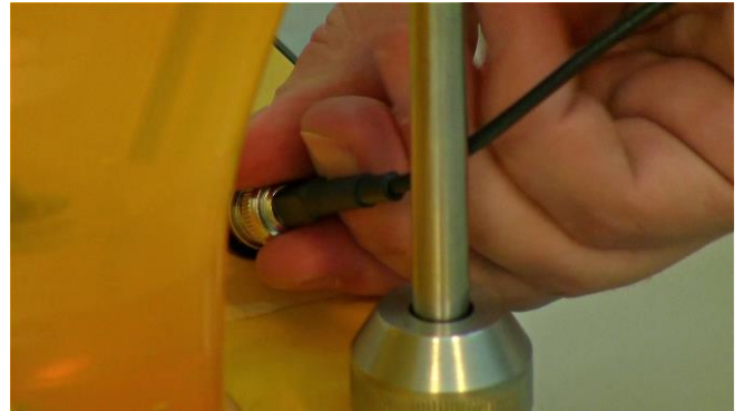
Figure 3.15—20 Secure the pO 2 (DO) probe connector into the socket by rotating and pressing to lock it together.
