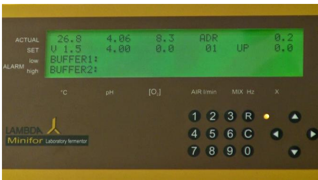
Figure 5.2—7 The pH of the buffer will be displayed on the ACTUAL value of the pH (above the SET value). Wait until the ACTUAL value of the pH gets stable.
