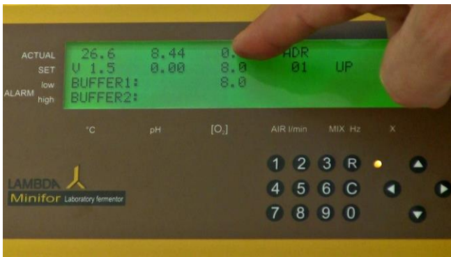
Figure 5.3—10 The ACTUAL reading for dissolved O 2 should always be '0' when the probe is disconnected. (If this is not the case then the probe may be faulty and you should check chapter Polarization, exchange of pO 2 Membrane / liquid, cleaning or contact the LAMBDA Helpdesk at support@lambda-instruments.com ).
