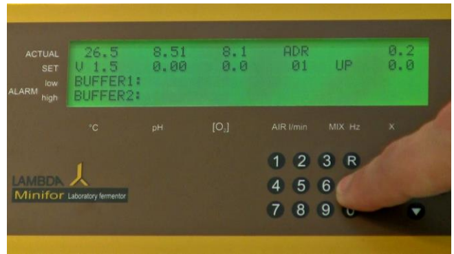
Figure 5.5—2 Long press of the calibration key "C" will activate the SET values on the display.
