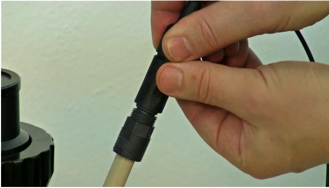
Figure 3.15—17 Place and adjust the pO 2 (DO) probe connector by rotating to find the position for exact locking of grooves with the pO 2 (DO) probe.
