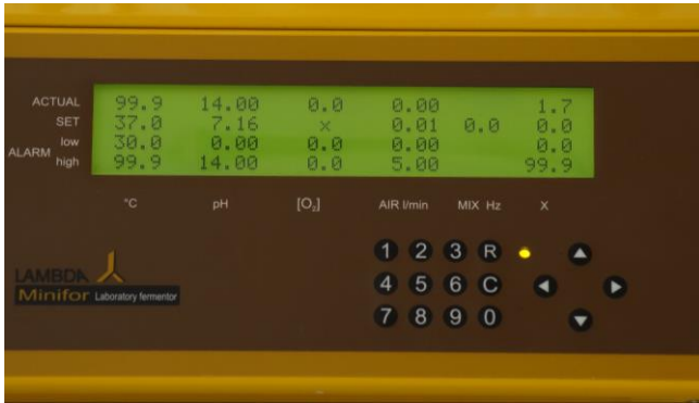
Figure 4.2—1 Standby mode - state of the fermenter after switching on. The display shows the last entered parameters. In this configuration all measurement readings are shown, but the regulation is switched off and the number keys blocked. LED is yellow and all numbers on the display are static.
