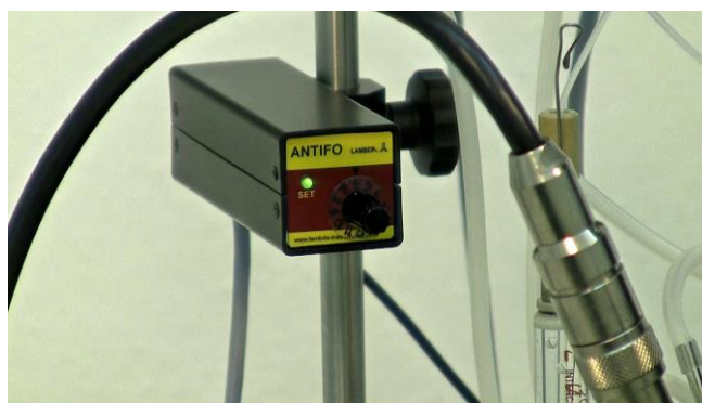
Figure 5.6—4 Sensitivity of the ANTIFO for the particular culture is now set. The LED will turn from green to yellow, when it controls the DOZITO for antifoam addition.
