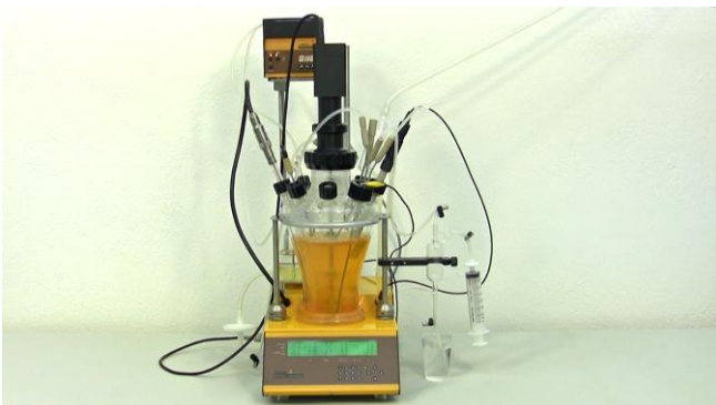
Figure 7.1—1 Fill 3/4th of the reaction vessel with buffer or medium.
