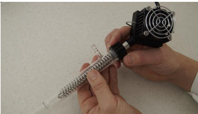
Figure 3.12-12 Insert the outgas condenser cylinder with the tubing connection over the condensing finger and tighten it securely by the black screw cap.
