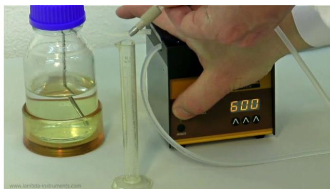
Figure 5.4—2 Turn the pump ON and have the other end of the tubing ready near the measuring cylinder. Carefully collect the liquid being pumped in the measuring cylinder for about 60 seconds.
