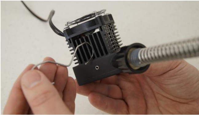
Figure 3.12-10 The attached peltier cell with the condensing finger should be made kept together with the help of the locking clamp.
