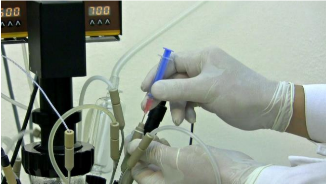
Figure 8.2—5 Remove the syringe along with its needle from the septum adaptor body.
