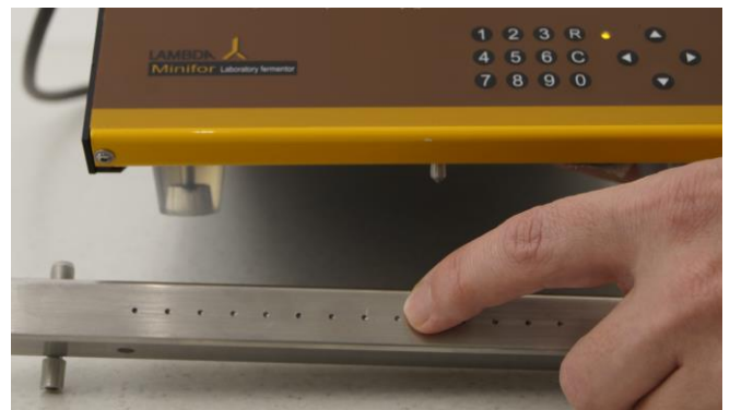
Figure 3.13—2 The steel tip (miniature scale module) under the front of the MINIFOR unit should be placed in these grooves of the weighing module.
