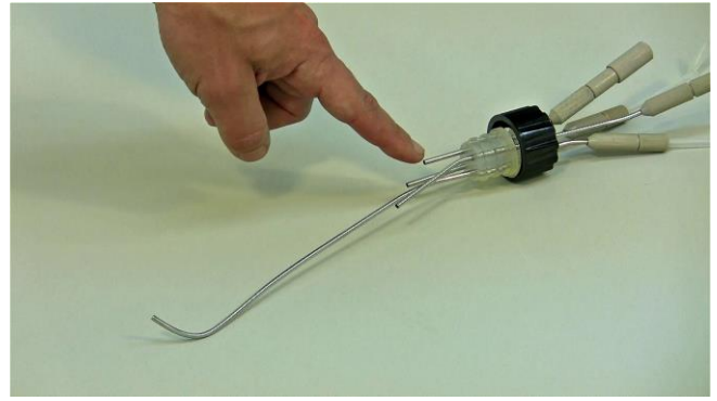
Figure 3.15—30 The second (foam) crocodile clip can be connected to any one of the three shorter needles of the quadruple sampling port.
