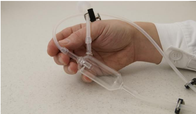
Figure 3.10-21 The tubing with the PEEK double-seal insert needs to be connected with the sterile sampling device. (Refer 3.10.2 Preparation of LAMBDA PEEK double seal connectors) Inlet provision for connecting the PEEK double-seal tubing has a provision tube deep inside the device glass part. (Please refer the picture)
