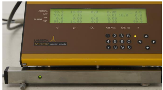
Figure 3.13—6 If the vessel weight is too low, an underscore sign “_” will appear along with the measured (actual) weight value [Refer Actual value of the parameter “X”] and a green LED light will be displayed in the weighing module.
