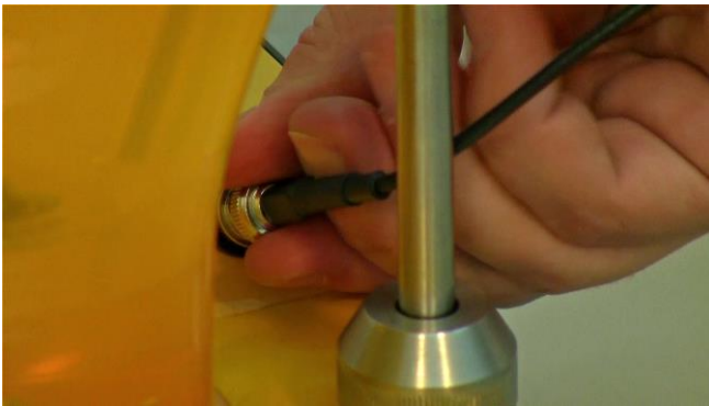
Figure 3.7-15 Secure the pO 2 (DO) probe connector to the socket by rotating and pressing to lock it together.
