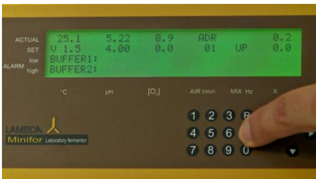
Figure 4.1—4 Press the "C" - calibration key continuously to activate the cursor.
