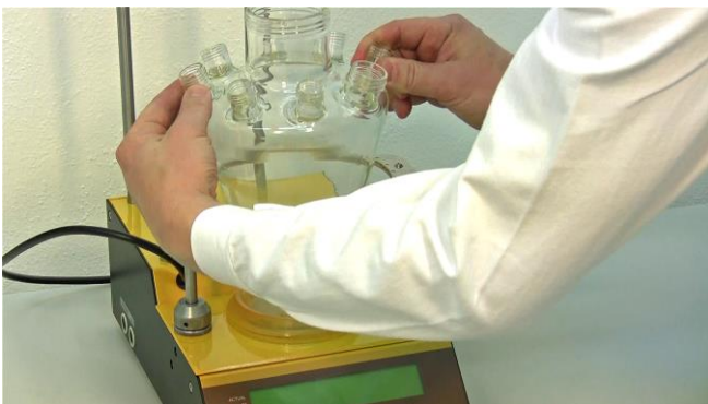
Figure 3.4-9 The port next to the quadruple port is the port usually defined for pO 2 Probe. The port just opposite to pO 2 probe is the port defined for pH probe. These ports for the probes are specially designed (placed nearly on the circumference of the vessel while the other ports are somewhat placed inside) to avoid the interference with the agitation unit.
