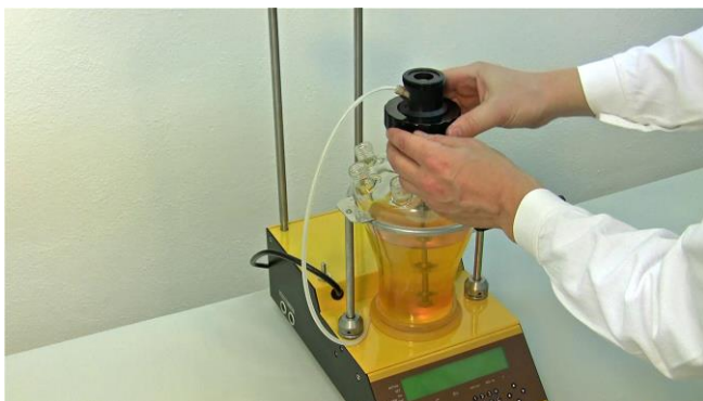
Figure 3.6-1 Take the free end of the air-input tubing (double seal connector tubing attached with mobile cock) from the head of agitation unit as shown.
