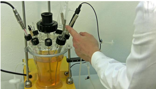
Figure 3.10-25 Remove the double-seal tubing protection closure on the longest cannula of the quadruple sampling port as shown.
