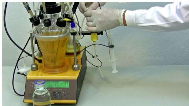
Figure 8.2—10 Pull the plunger of the syringe to fill the sampling glass device with the sample from the reaction vessel. Never fill the glass device completely. If the sample is needed in large amount, it can be sampled twice. Close the clamp on the sampling inlet. Open the clamp on the outlet.
