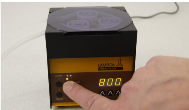
Figure 3.16—12 LED illumination in the direction \blacktriangleleft represents the clockwise rotation.
