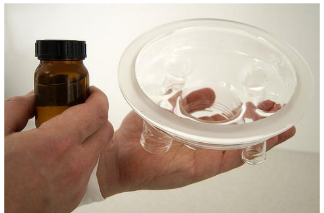
Figure 3.4-26 Apply a small amount of silicone oil on the vessel upper part's brim for easy removal of the parts after completing the experiment.
