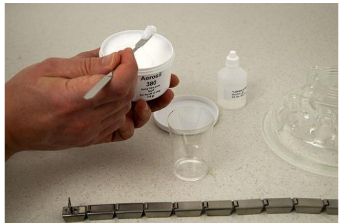
Figure 3.4-22 Take equal parts of solution A and solution B in a non-glass beaker. For example: 2g of Solution 'A' and 2g of Solution 'B'. Aerosil powder is added in such an amount until the mixture is no more flowing.
