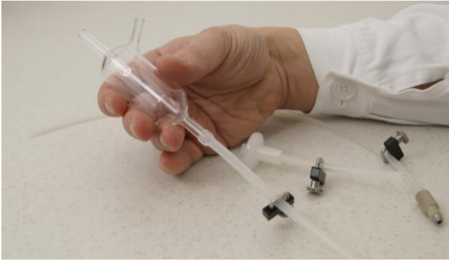
Figure 3.10-19 Silicone tubing which is 10 - 20 cm long needs connected to the output arm provision on the glass device i.e. the vertical arm opposite to the inlet sampling connection with the Bioreactor (on the lowest part of the device)
