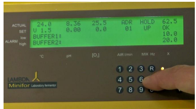
Figure 5.5—12 Wait until the message “HOLD” appears and then press the calibration key “C”. The message “OK” will appear indicating that the calibration has been accepted by the MINIFOR fermentor unit. Now, the scale is calibrated in g or ml. Weight calibrations can be made according to your need with weights.
