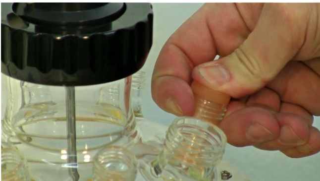
Figure 3.7-5 Insert the coloured rubber stopper for the pO 2 (DO) probe on the right side of the port which is next to the sampling port (larger in diameter)
