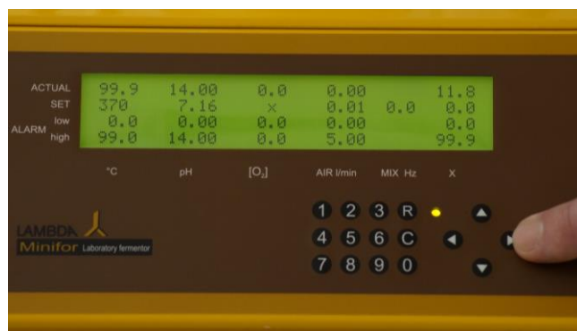
Figure 4.3—2 Enter the value for the desired temperature (the value shown on the first line and first column corresponds to the measured temperature and cannot be changed).
