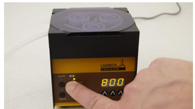
Figure 3.16—13 LED illumination in the direction \blacktriangleright represents the anticlockwise rotation.
