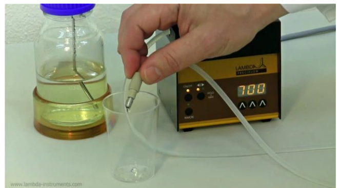
Figure 5.4—9 Carefully collect the liquid being pumped into the measuring beaker for about 60 seconds.
