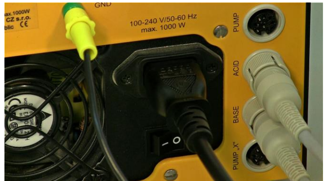
Figure 3.15—43 Connect the Power cord to the power inlet (100-240 V/ 50-60 Hz) at the rear of the MINIFOR base control unit.
