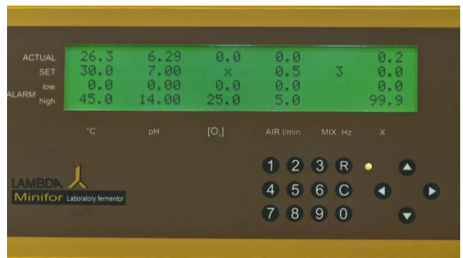
Figure 5.3—17 The 'ACTUAL' reading should show '0' after stabilization.
