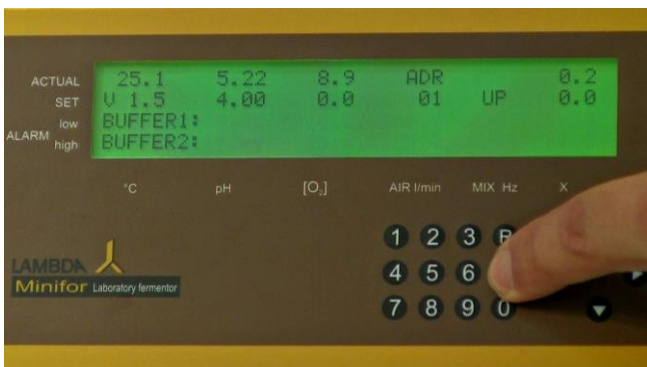
Figure 5.2—3 Continuous pressing of "C" key will activate the cursor of the set value of pH.
