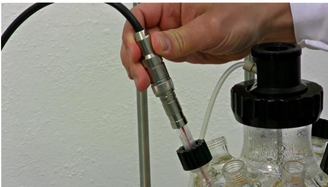
Figure 3.15—7 Connect both the pH probe connector and cable from the MINIFOR base unit with the pH probe. Rotate and adjust the connector cable for exact locking of grooves.
