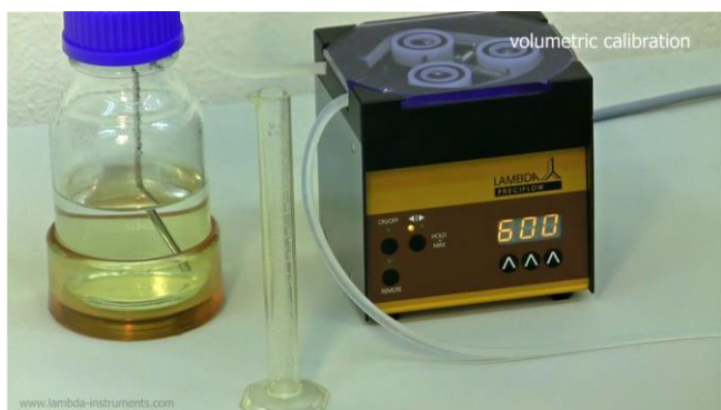
Figure 5.4—1 Connect the tubing to liquid in the bottle and set the desired speed (e.g. 600). Keep the measuring cylinder ready.
