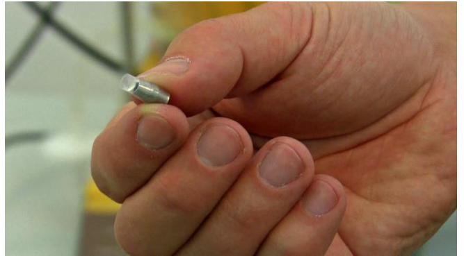
Figure 3.10-12 The tubular septum (which is sealed at one end) should be fitted over the double seal conical insert with the use of, for example, a hard ruler leaving part of the tubular septum free and exposed as shown.
