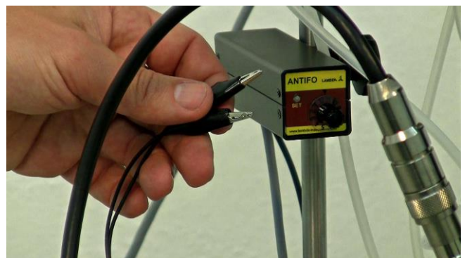
Figure 3.14—2 The two crocodile clips of the ANTIFO need to be connected with the cannulas from the quadruple sampling port for the detection of the foam level in the working vessel.
