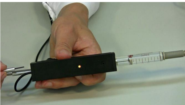
Figure 5.6—9 When the DOZITO receives the signal from ANTIFO, the LED will be illuminated as yellow and the pusher rod will push the syringe's plunger and thus delivers the pre-set volume of antifoam agent.
