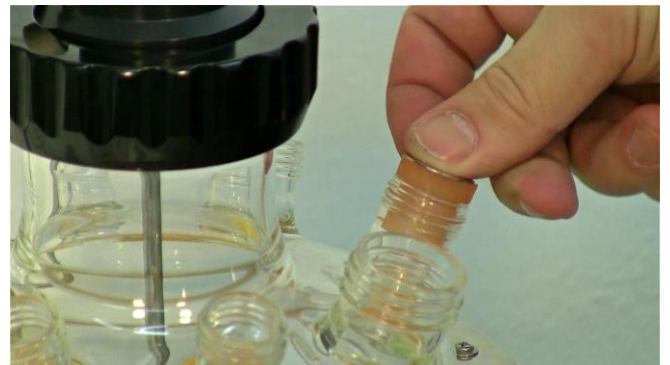
Figure 3.7-6 Make sure the washer is placed on to the rubber stopper.
