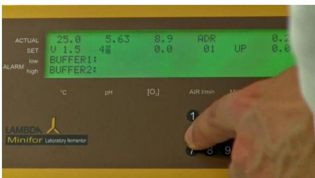
Figure 4.1—7 The number key is used to change the value of the blinking cursor.
