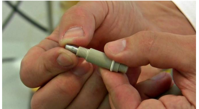
Figure 3.10-14 Note that the sealed end of the tubular septum should be fitted into the septum adaptor body (on the other side of white septum O-ring) such as shown.
