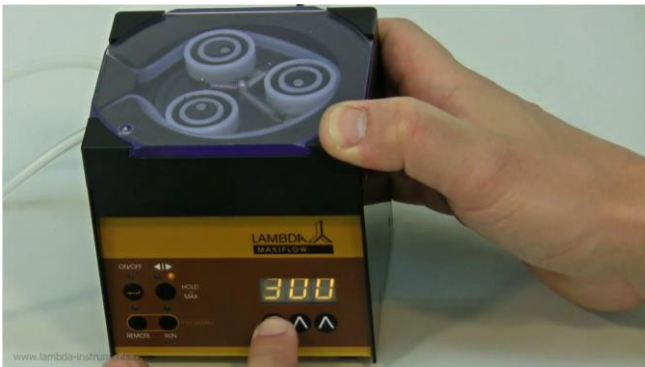
Figure 3.16—10 The \wedge \wedge \wedge buttons can be used to set the desired flow rate.
