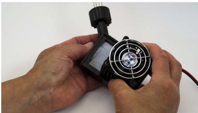
Figure 3.11-7 Detach the motor and fan unit from the cooling pipe as shown while preparing for sterilization.
