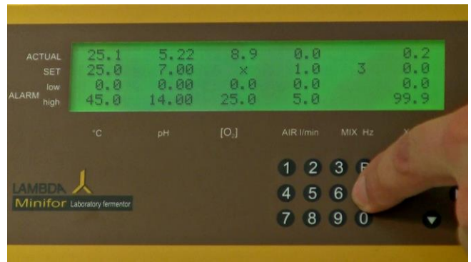
Figure 5.2—2 Change the stand-by mode into calibration mode by pressing the calibration key "C".
