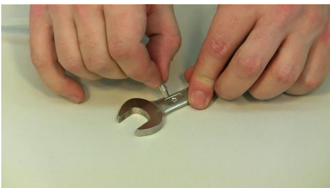
Figure 3.5-9 Take a spanner and the double seal conical insert with the tubing. Press the conical insert with the tubing against the spanner to make it inserted totally into the tubing.
