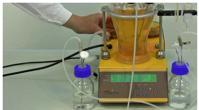
Figure 7.1—10 Store the magnetic bottle holders at the back of the main base control unit.
