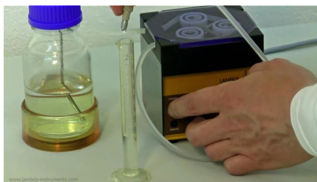
Figure 5.4—4 Exactly after 60 seconds, switch OFF the pump.
