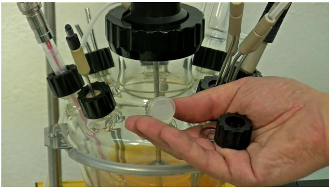
Figure 7.1—3 Fit the closed stopper with metal washer and a screw cap on the unused side necks in the vessel.
