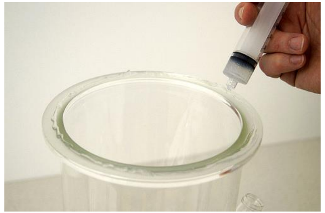
Figure 3.4-24 Apply the mixture on the whole circumference of the lower vessel part's brim like a "spaghetti".
