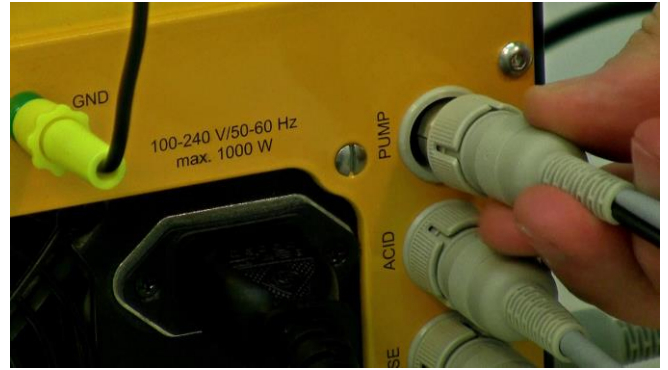
Figure 3.16—19 Other additional pumps can be connected to the PUMP socket.
