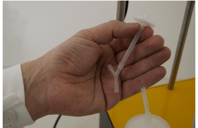
Figure 3.6-10 Add a Y-piece into the aeration tubing.
