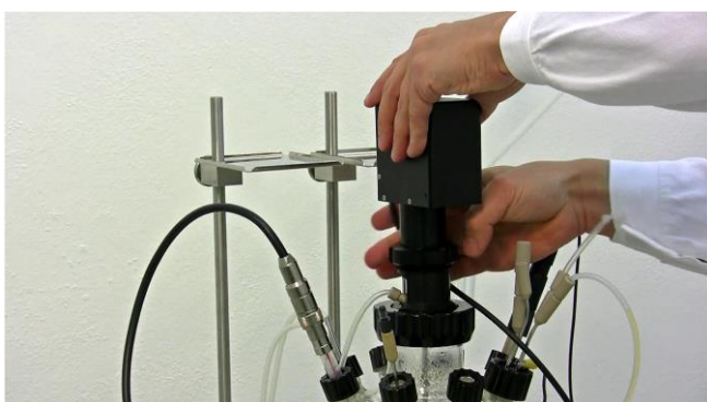
Figure 3.15—3 Once the magnets are engaged, the air-input with the mobile PEEK cock displace downwards. Secure the vibromixer firmly by screwing the cap.
