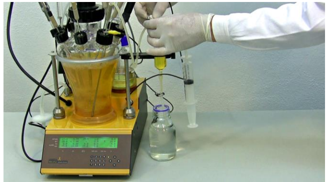
Figure 8.2—4 Close the clamp on the inlet tubing to avoid the back flushing of the sample into the reaction vessel.
