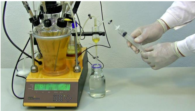
Figure 8.2—3 Pull the plunger of the syringe to fill the sampling glass device with the sample from the reaction vessel. Never fill the glass device completely.
