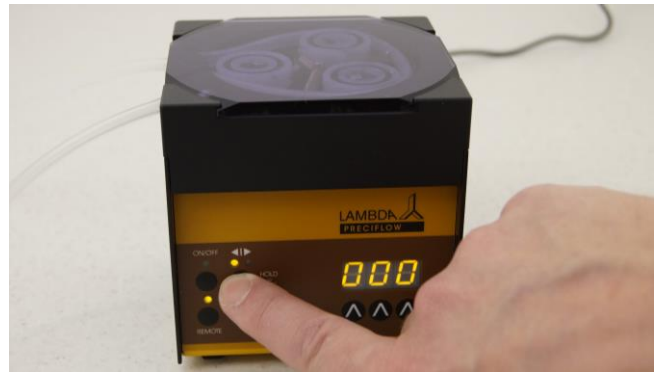
Figure 3.13—9 Press the remote button on the connected 'X'-channel Peristaltic pump.
