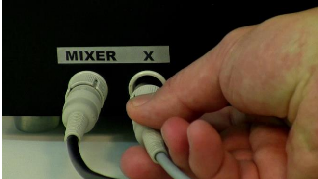
Figure 3.13—3 Connect the weighing module connection cable in the "X" socket beside the "MIXER" on the left side of the MINIFOR base control unit.
