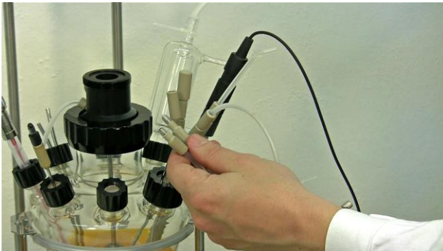
Figure 3.10-27 Take the prepared tubing with the PEEK double-seal tubing connectors at both the ends of the tubing (Refer 10.3.2 Preparation of PEEK double-seal tubing connectors).
