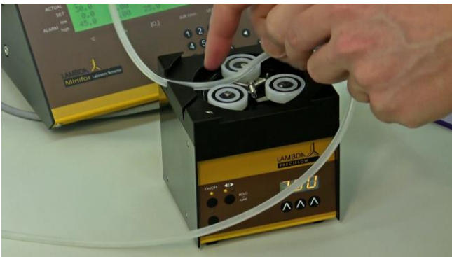
Figure 7.1—13 Remove the acid and base tubing lines from the Peristaltic Pumps.
