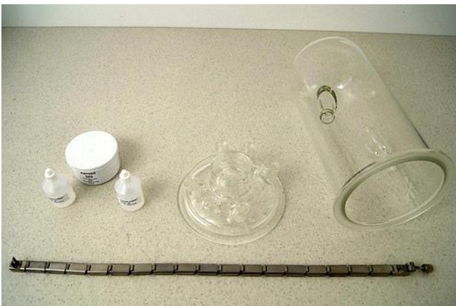
Figure 3.4-21 Get ready with the reaction vessel, Liquid O-ring ingredients and the closing belt.
