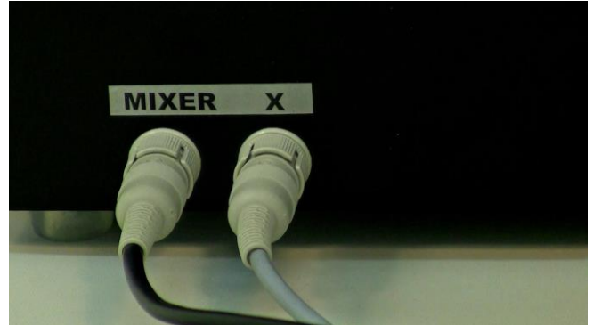
Figure 3.13—4 Insert the plug and tighten it securely by screwing the adjustable sleeve present in the plug.
