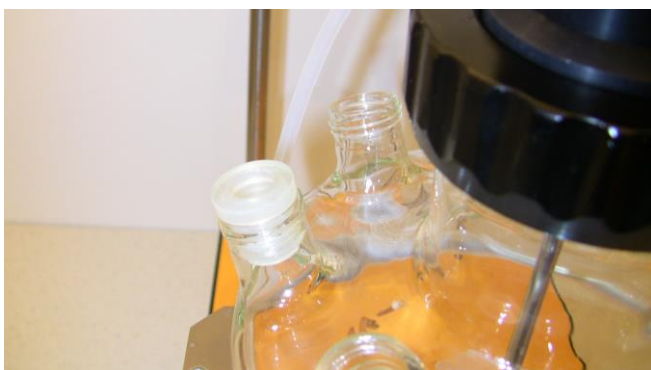
Figure 3.8-3 Place any one of the provided white open stopper on the port which is opposite to the pO 2 probe port.
