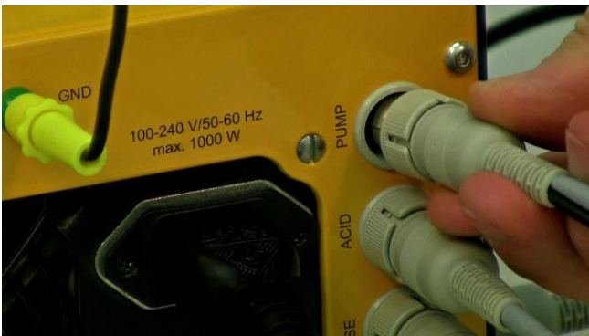
Figure 3.15—23 Peltier outgas condenser can be directly connected on the “PUMP”socket present at the rear of the MINIFOR base control unit.
