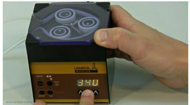
Figure 3.16—11 Each \wedge \wedge \wedge arrow can be used to change the corresponding digit on the flow rate.
