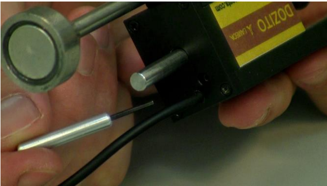
Figure 5.6—5 Use the key given with the ANTIFO and DOZITO kit for setting up the volume of the anti-foam agent added.
