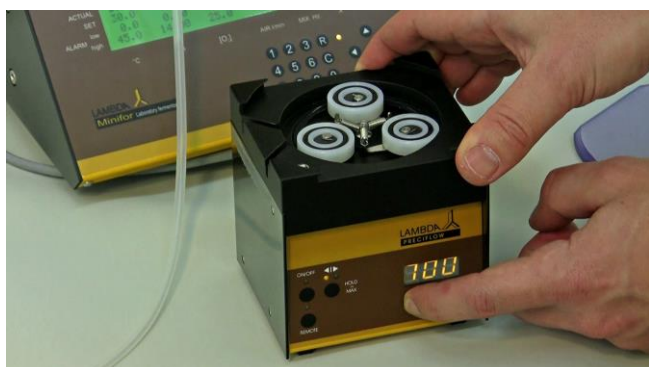
Figure 3.16—3 Set the pump speed to about 700. The speed range of about 300-700 for tubing insertion can be used.
