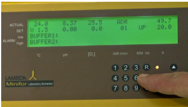
Figure 5.5—14 To change the pump regulation, press the calibration key "C" to change the standby mode to calibration mode.
