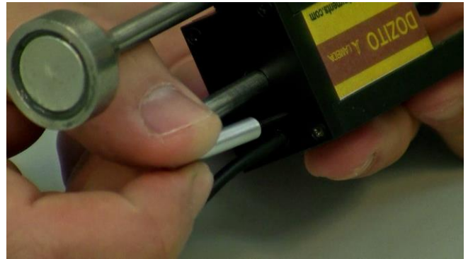
Figure 5.6—6 Insert the key at the insert point next to the pusher rod.
