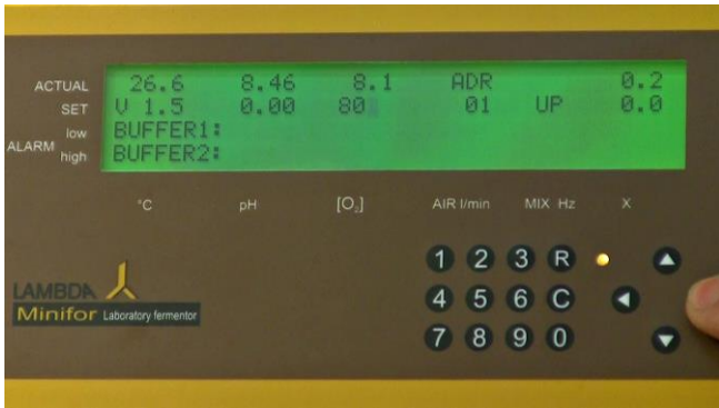
Figure 5.3—5 Enter the value from the table in the SET [O 2 ] and then press the right arrow key (>). (e.g.: 80)
