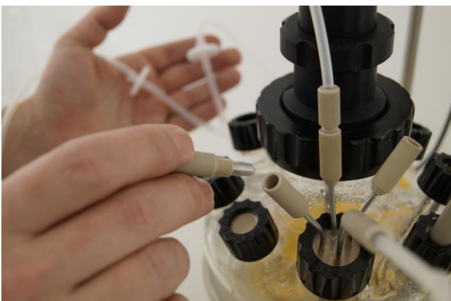
Figure 3.6-13 Connect the tubing for surface aeration to the hollow small cannula in the quadruple sampling port that stays in the head space of the MINIFOR above the medium surface.
