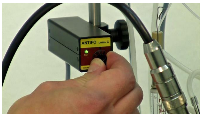
Figure 5.6—3 Now rotate the knob anticlockwise (about 1mm) to set the sensitivity point and the LED displays green i.e. the point at which yellow turns to green.
