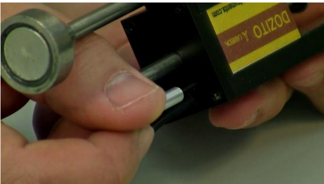
Figure 5.6—7 Screwing in = clockwise rotation = decrease of the delivered anti-foam volume / step
