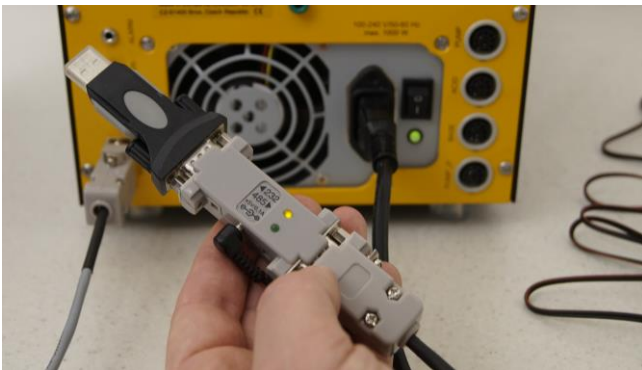
Figure 6.4—5 Illuminated LED indicates that the converter is ready to operate.
