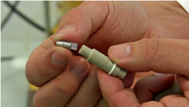
Figure 3.10-13 The prepared double seal conical insert with the tubular septum has to be inserted into the septum adaptor body.
