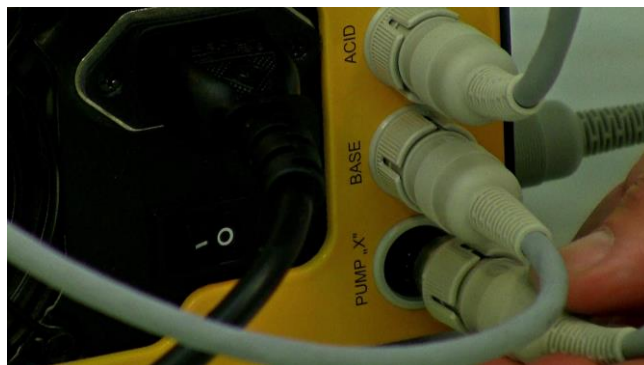
Figure 3.15—26 Connect the corresponding pump (for the addition or removal of medium) to the “PUMP X” socket on the rear of fermenter-bioreactor MINIFOR.
