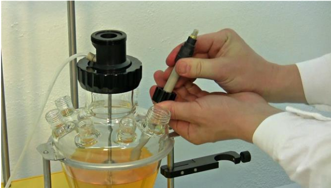
Figure 3.7-9 Insert the probe through the fixed coloured stopper and screw cap. Then, push the probe carefully into the port and adjust the height of the probe to be immersed in the medium
