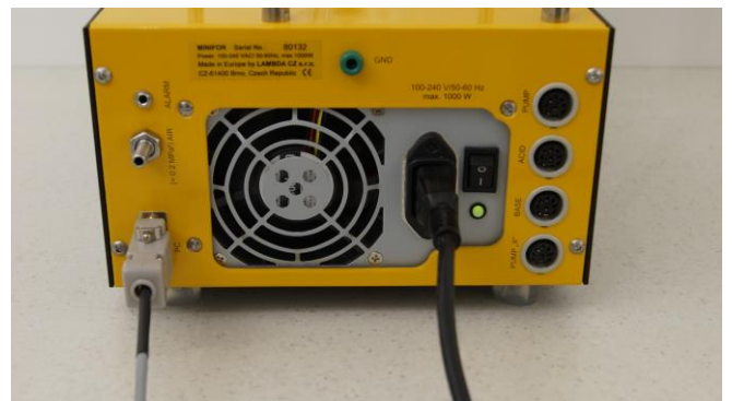
Figure 3.15—41 The alarm connector cable plug has to be connected into the alarm socket at the rear of the base control unit. Other end of the cable can be connected to the desired devices.
