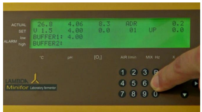
Figure 5.2—8 Once the ACTUAL value of the pH is stable, press the calibration key "C" in order to save the calibration. The calibrated value will be displayed as BUFFER 1 value of pH.
