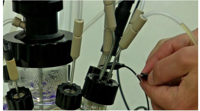
Figure 3.14—4 Connect one of the crocodile clips to the harvest needle of the quadruple sampling port.
