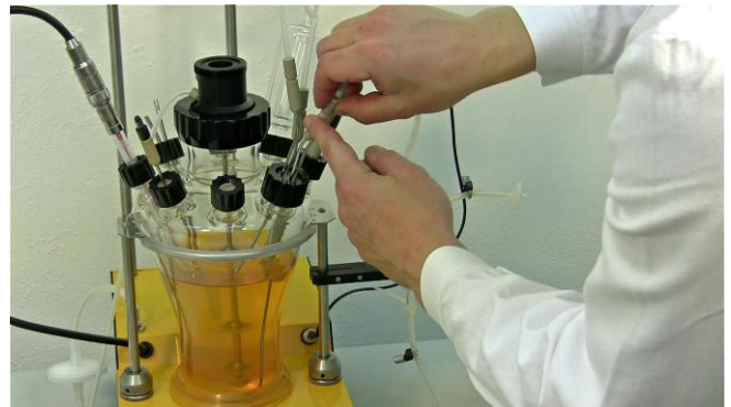
Figure 3.10-26 Take the PEEK double-seal tubing from the sterile sampling device and connect it with the longest cannula on the quadruple sampling port.
