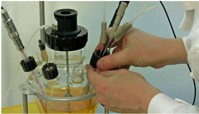
Figure 3.10-23 Insert the quadruple sampling assembly into the port which is larger in diameter and adjacent to pO 2 probe set-up. Fix and tightly secure it with the black screw cap.
