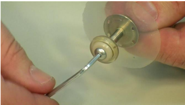
Figure 3.5-23 The key tightening of the self-cleaning microsparger at the end of the sparger pipe.
