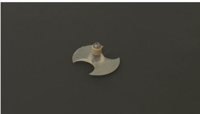
Figure 3.5-27 Butterfly-shaped stirrer disc for the 0.3L vessels.
