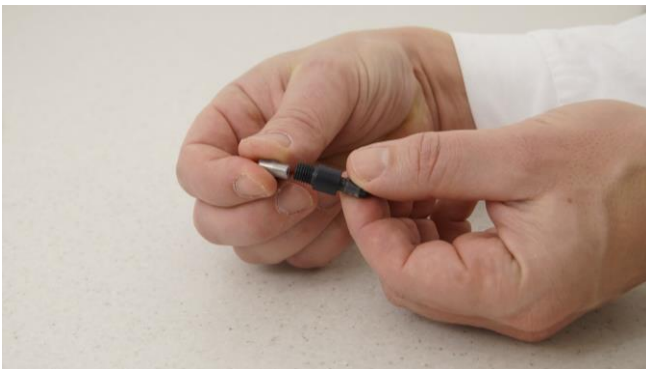
Figure 3.9-1 Insert one end of the double-conical tubing insert to the over pressure security valve.
