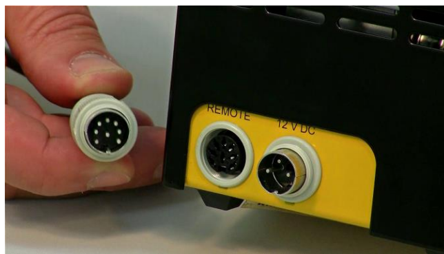
Figure 3.15—12 Connect one end of the remote control cable to the corresponding “REMOTE” sockets at the rear of the peristaltic pump or MASSFLOW.
