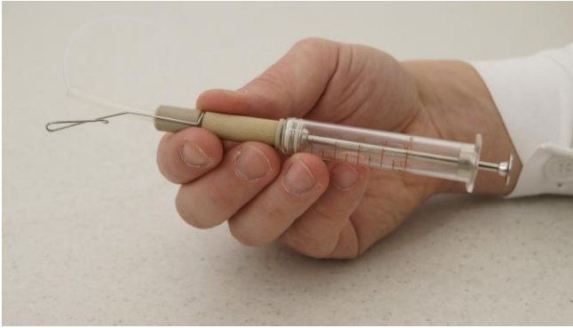
Figure 3.14—11 Prepared sterilizable syringe with the antifoam line.
