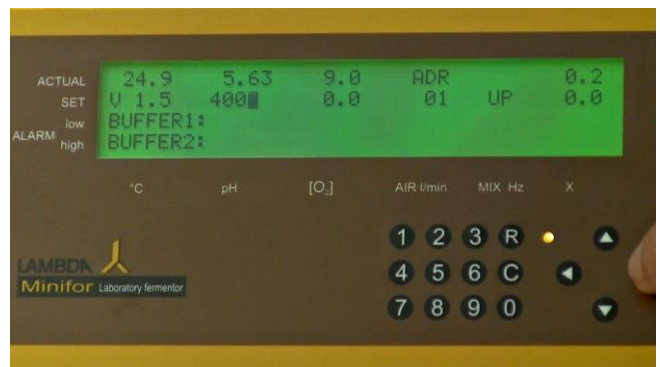
Figure 5.2—4 To start the gauging of the first pH, enter the desired pH as the set value using the number keys.
