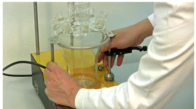
Figure 3.4-10 Adjust the deeply inserted reaction vessel holder around the reaction vessel so that it is supported well. This may be a little stiff, so please be careful.
