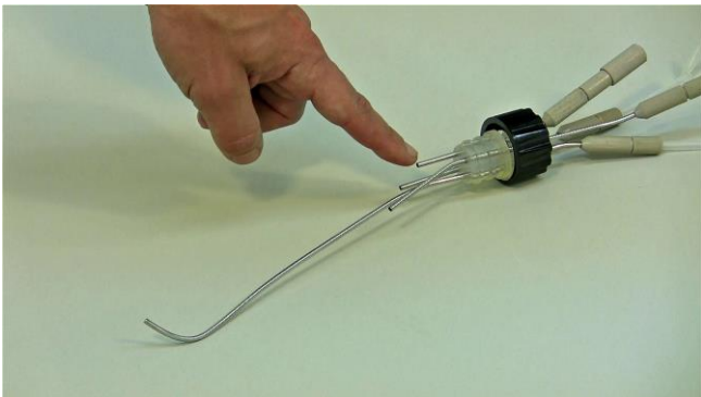
Figure 3.14—5 The second (foam) crocodile clip can be connected to any one of the three shorter needles of the quadruple sampling port.
