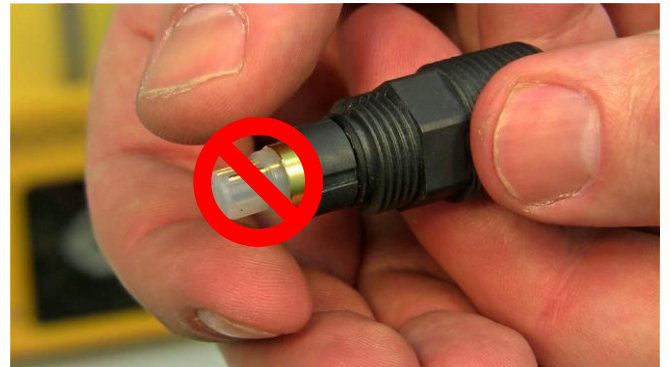
Figure 3.7-4 Please be careful not to touch this part of the probe.
