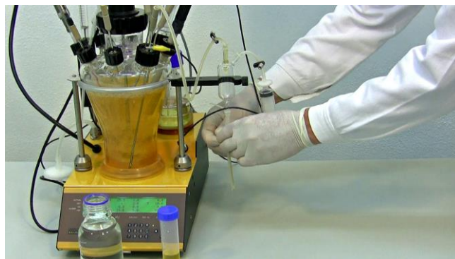
Figure 8.2—12 Close the clamp on the outlet tubing.
