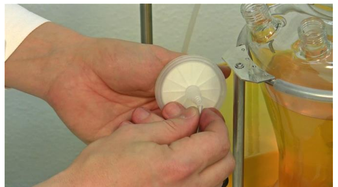
Figure 3.6-2 Connect the air-input tubing from the agitation unit to one end of the air-input filter.
