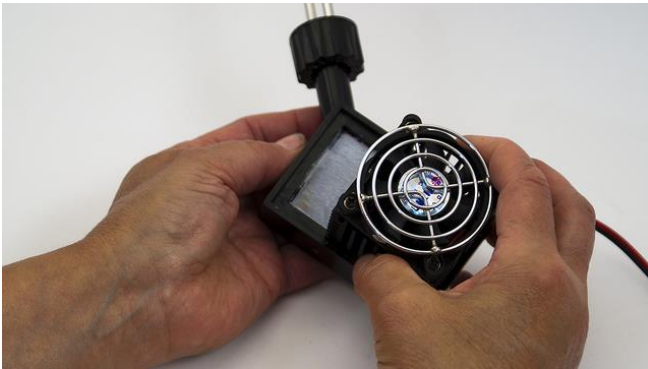
Figure 3.11-11 Attach the Peltier cooling element with control electronics and fan with the cooling loop by placing the white surface with the heat-conductive paste onto the respective trap in the cooling finger attachment as shown.
