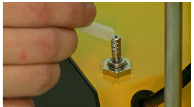
Figure 3.6-6 With the other end of the tubing from the air-input filter, connect it to the air outlet on the base control unit as shown. Insert the tubing deeply till the bottom of the air outlet.
