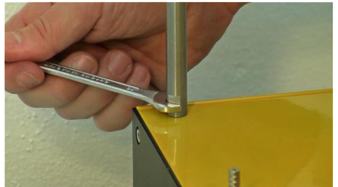
Figure 3.3-2 Further fix the inserted support rod tightly with the supplied spanner.
