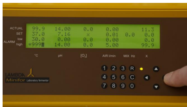
Figure 4.3—4 Move the cursor on the field of temperature maximum (ALARM HIGH). Enter the desired value. If the temperature exceeds this value, an alarm is activated and the exceeded value is highlighted on the display.
