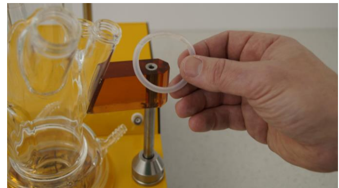
Figure 3.4-16 Place the reaction vessel on the base unit with which the distinct side arms for pH and pO 2 probes are supported by the lateral reaction holders. The elastic silicone ring helps to affix the vessel with the reaction holder.
