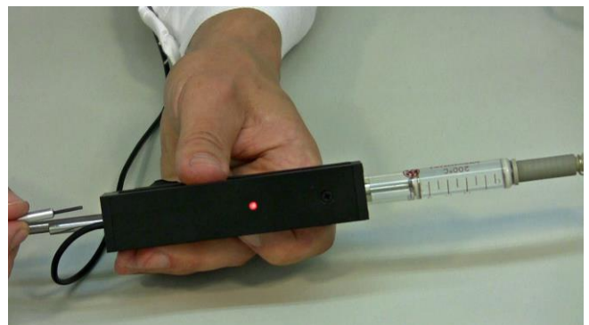
Figure 5.6—10 When the preset dose has been delivered, the LED will switch to red. Then the communication with ANTIFO is interrupted for approximately 20 seconds and the indicator LED is turned off.
