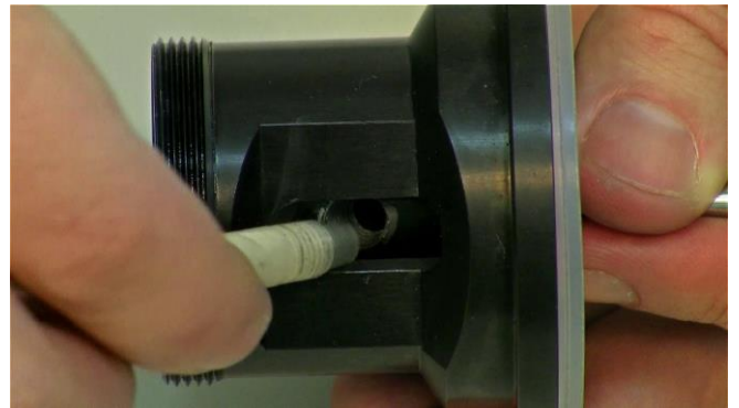
Figure 3.5-18 Insert the prepared double-seal tubing connector into the mobile cock through the head of agitation unit. Screw the double-seal tubing connector clockwise to tighten it.
