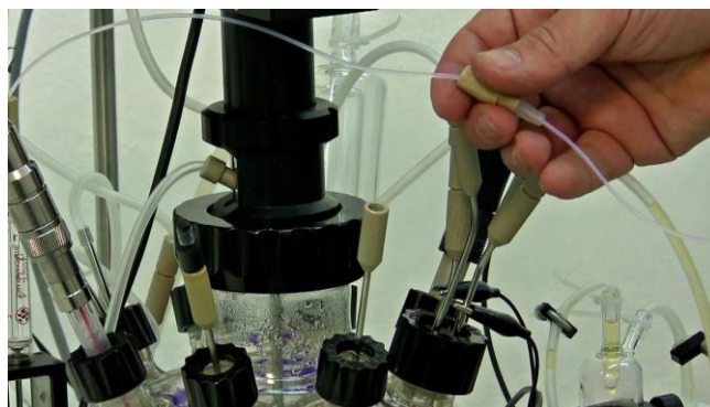
Figure 3.14—26 The PTFE antifoam line has to be connected with the shortest cannula that will facilitate the addition of antifoam above the liquid level.
