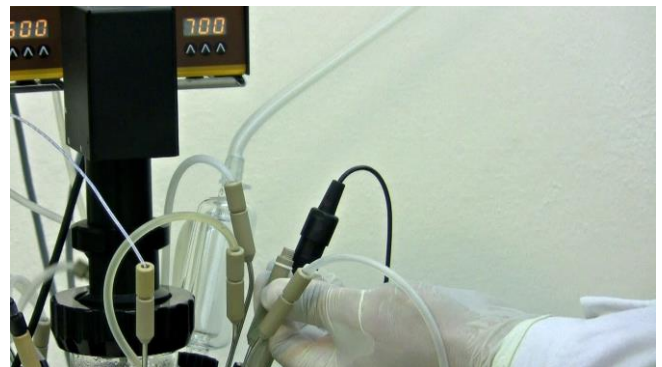
Figure 8.2—2 Remove the septum protection cap completely and get ready with the inoculum / inoculant.
