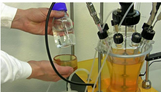
Figure 7.1—9 Remove the magnetic bottle holders from the storage bottles.
