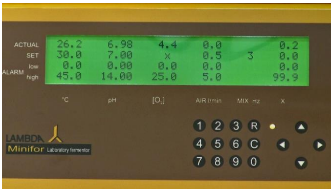
Figure 4.1—1 Stand-by mode of the MINIFOR. “R” key used to switch between Standby and Regulation state (RUN with REGULATION)
