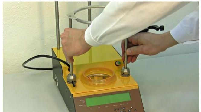
Figure 3.4-6 The vessel reaction holder with the sterile sampling device holder needs to be fixed on the MINIFOR base control unit. Place the reaction vessel holder in the 2 desired slots on either side of the sun-like heating element.
