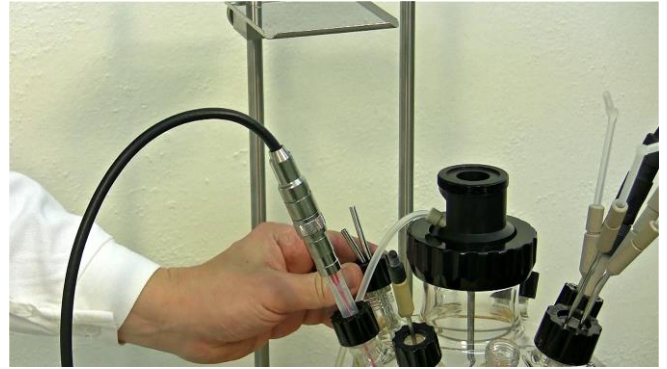
Figure 3.11-4 Secure and fasten gently with the black screw cap.
