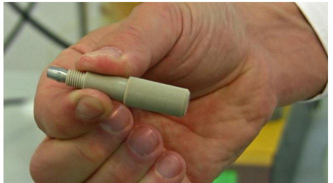
Figure 3.10-16 Complete set for inoculation. The free end with the double seal conical insert has to be inserted on one of the cannulas or needles from the quadruple sampling port.
