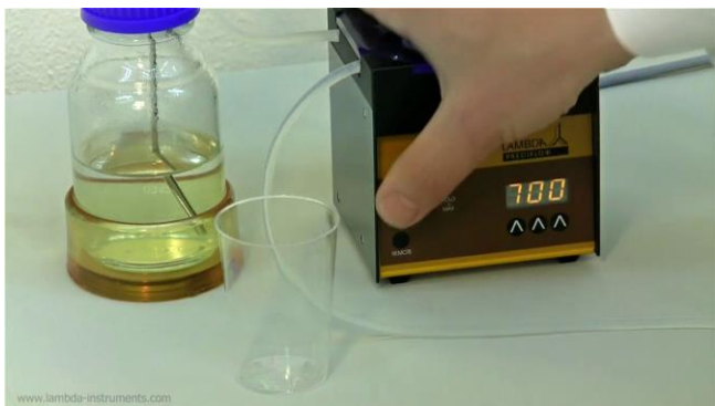
Figure 5.4—8 Switch the pump ON and have the other end of the tubing ready near the measuring beaker.
