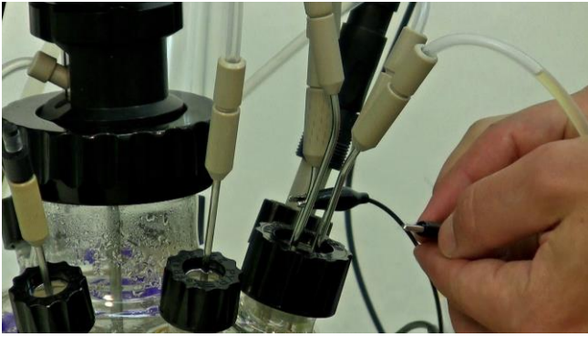
Figure 3.15—29 Connect one of the crocodile clips to the harvest needle of the quadruple sampling port.
