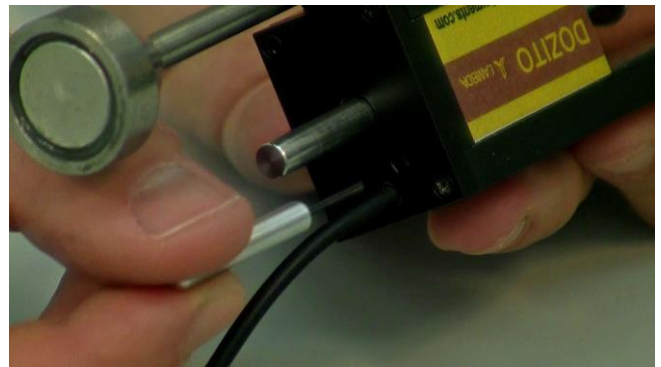
Figure 5.6—8 screwing out = counter-clockwise rotation = increase of the delivered antifoam volume / step
