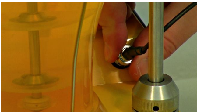
Figure 5.3—8 For the Zero point calibration, disconnect the pO 2 (DO) probe from the socket in base control unit.
