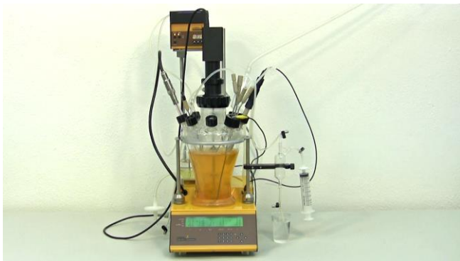
Figure 5.3—1 After the polarization, the pO_2 probe has to be calibrated before and after sterilization. pH/Pt 100 probe should be inserted during calibration.
