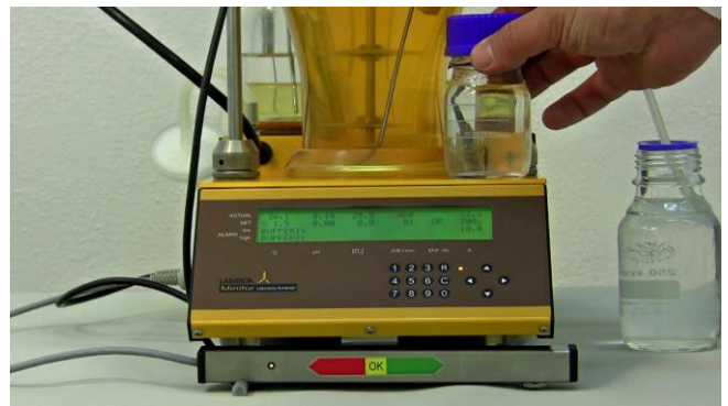
Figure 5.5—6 Place a known weight on the MINIFOR base control unit. For example, place an empty glass bottle.
