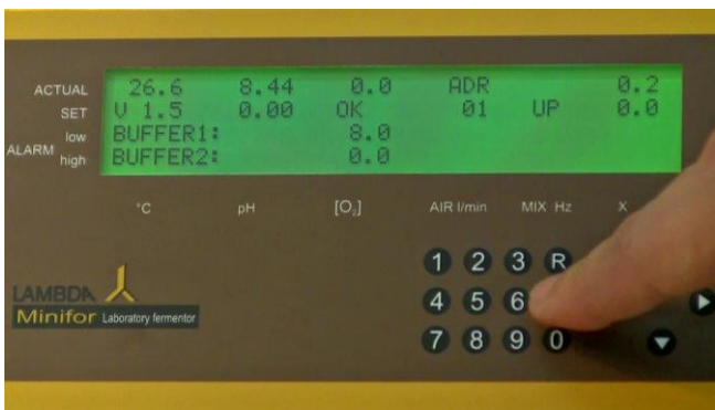
Figure 5.3—12 Press the calibration key "C". The calibrated value will be saved and displayed as BUFFER 2 value of [O 2 ]. OK message will be displayed if the calibration done correctly.
