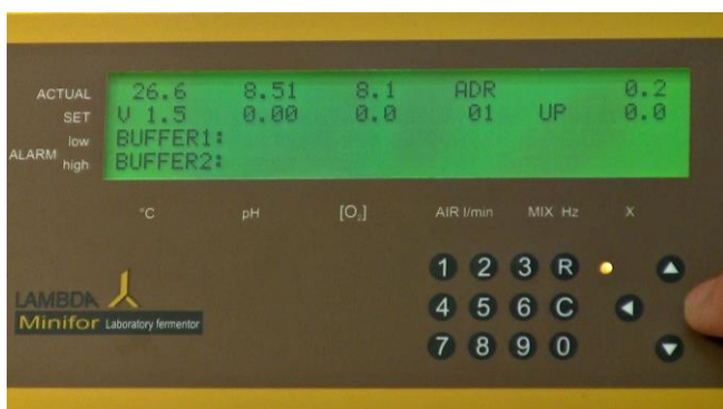
Figure 5.3—3 Move the cursor to the [O_2] value using the right navigation key (>).
