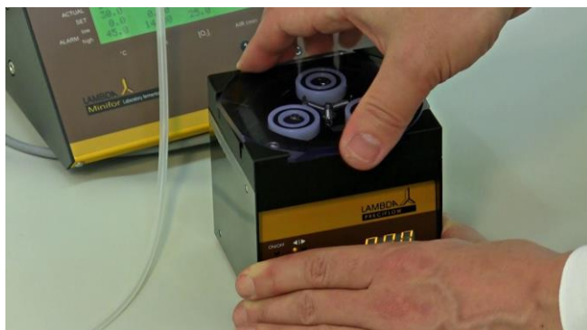
Figure 3.16—1 For the installation of tubing into the Peristaltic pump, twist the transparent PVC head cover either clockwise or anti-clockwise to remove.
