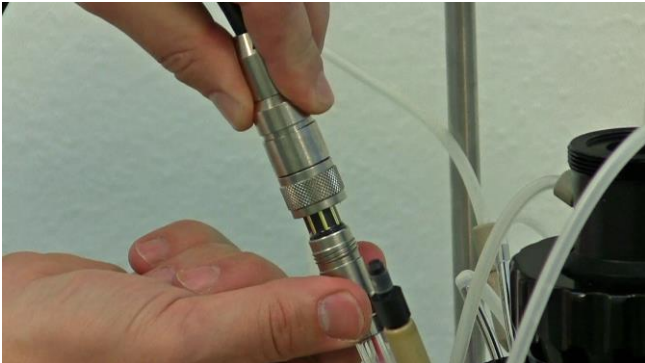
Figure 7.1—7 Disconnect the pH probe connector from the pH probe.
