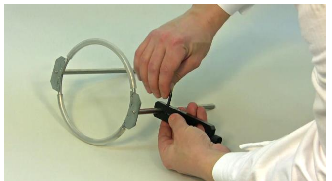
Figure 3.4-4 After inserting the sterile sampling device holder and positioning it, fix the corresponding screws as shown with the given key to make it hold firmly.
