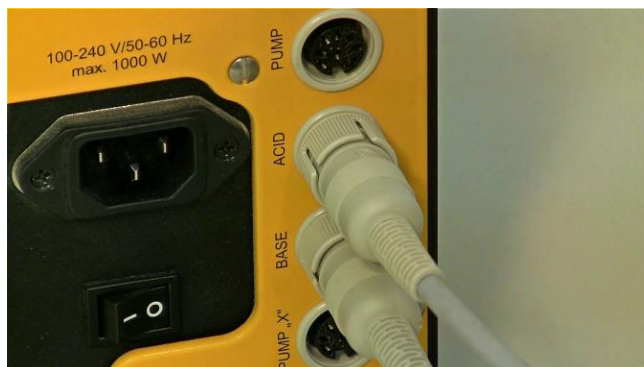
Figure 3.15—14 Connect the Peristaltic pump that regulates the acidity of the reaction to the “ACID” socket at the rear of the MINIFOR base control unit.
