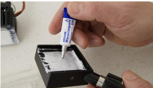
Figure 3.12-8 Apply the heat-conductive paste on the white surface of the Peltier cooling element with control electronics and fan, before attaching the condensing finger with the unit. Spread out the heat-conductive paste on the surface evenly and thinly ensuring that there are no trapped air bubbles.
