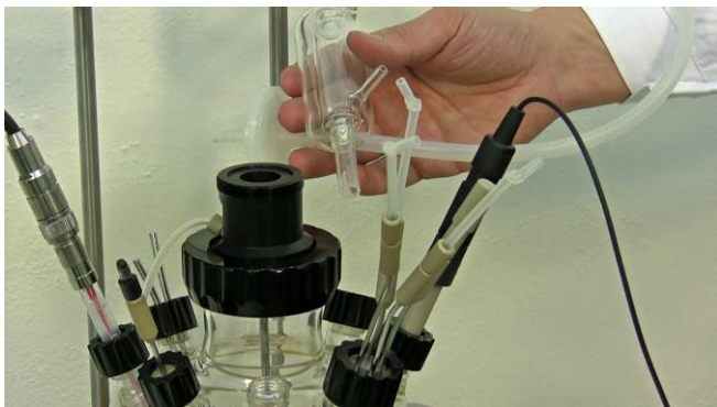
Figure 3.12-2 Glass outgas condenser and gas outlet filter need to be sterilized together with the MINIFOR vessel.
